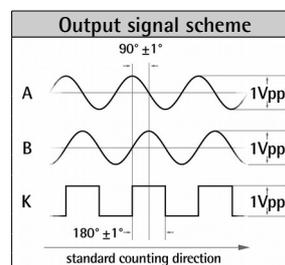
1 K Index signal, see the order code, with N code the signal is not provided
