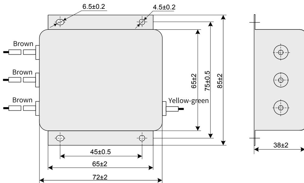
Figure 12-7 Dimensions of the safety capacitance box
