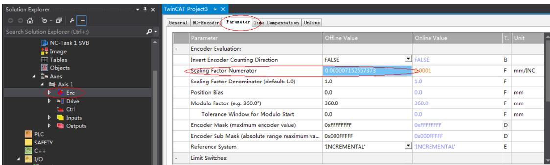
■ **Scaling factor Numerator:** Indicates the distance corresponding to the encoder pulses per position feedback.
