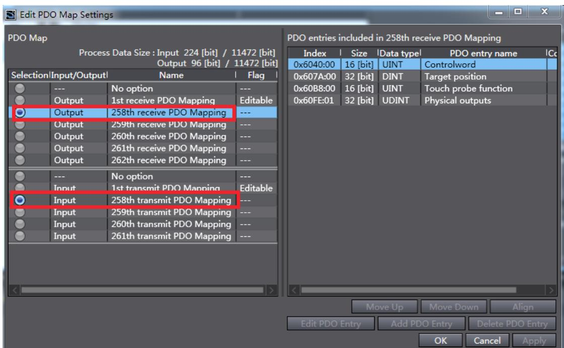
Modify the PDO mapping object through **Add PDO Entry** and **Delete PDO Entry**. The frequently used mapping parameters are shown below.
