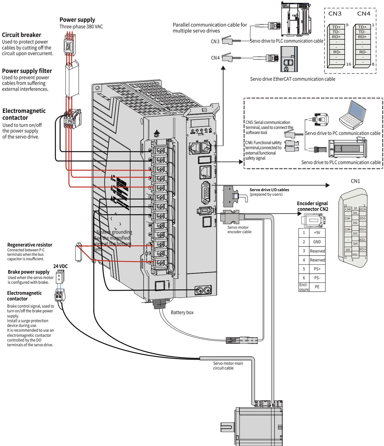
Figure 1-15 Wiring of three-phase 380 V servo systems
