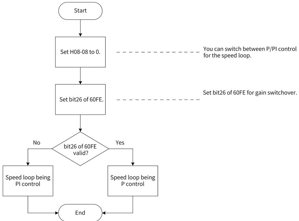
Figure 6-6 Gain switchover flowchart (H08-08 = 0)
