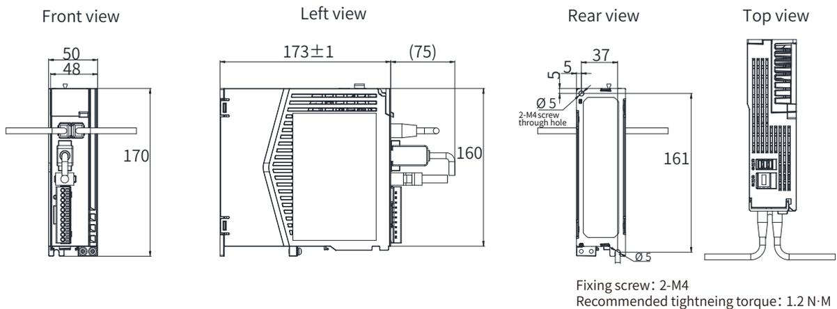
Figure 2-2 Outline dimensions of size B (unit: mm)
