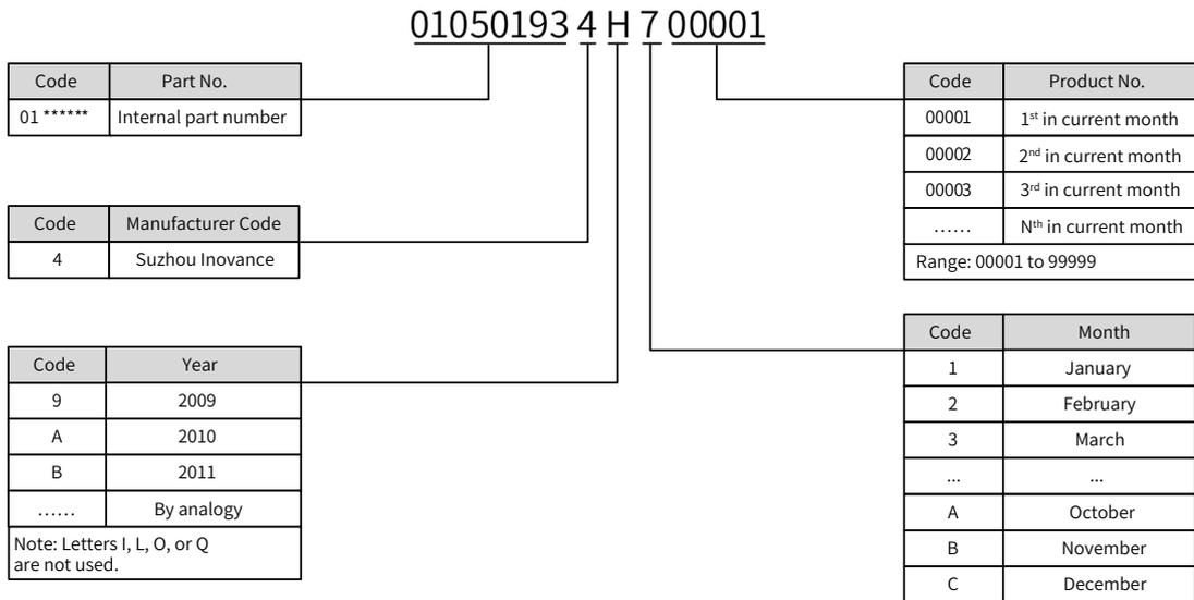
Example: The serial number 010501934H700001 indicates the servo drive is manufactured in July 2017.
