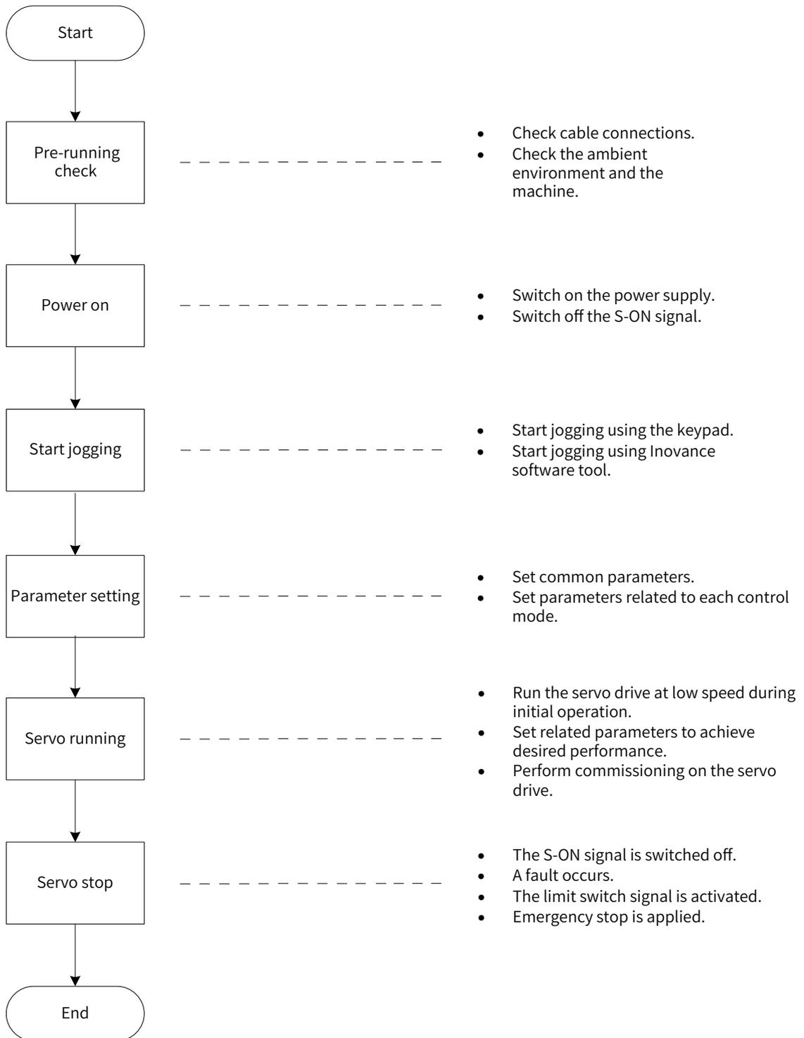
Figure 5-1 Flowchart for setting the servo drive
