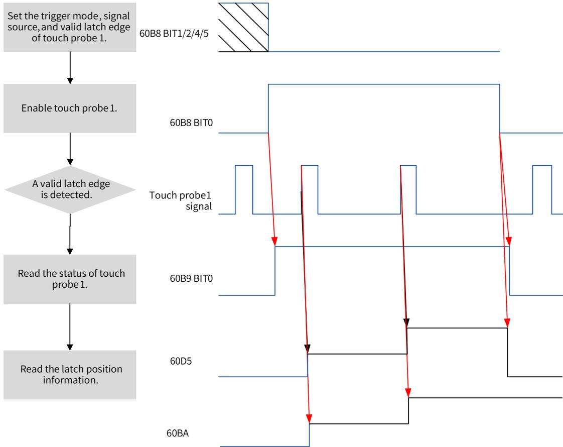
Figure 7-84 Operating procedure of touch probe function
