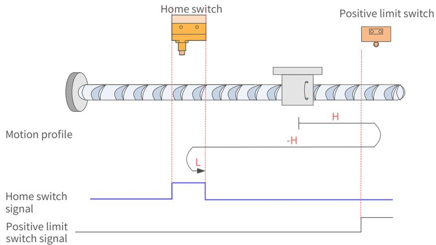
Figure 7-70 HW signal inactive at start, hitting the positive limit switch
