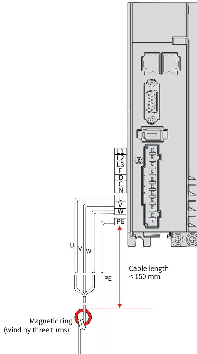
Figure 12-8 Installation of the output magnetic ring (external)
