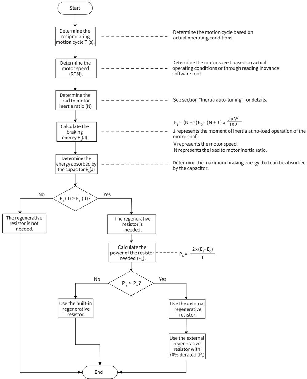
Figure 5-7 Flowchart for selecting the regenerative resistor
