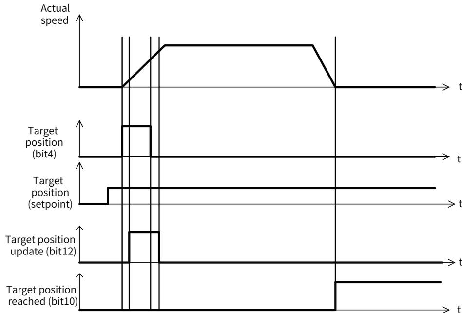
The linkage mode of position references is determined by bit5 (Change set immediately) of the control word. When bit5 is set to 1 (Sequential mode), sequential linkage applies between position references. When bit5 is set to 0 (Single-point mode), linkage applies between position references after reaching zero speed.
