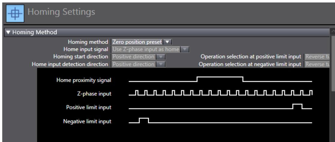
The homing mode involves the servo drive and the host controller. Set the homing mode according to the following table.
