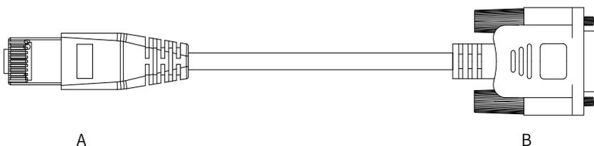
Figure 3-24 Outline drawing of the PC communication cable
