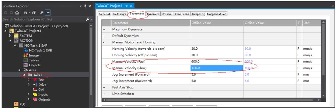
7-2) Controlling the servo operations through the PLC
