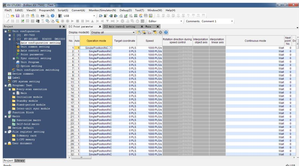
2. Move the mouse to the point parameter, such as No.1-Axis1, and wait until the mouse icon to change from an arrow to a small hand. Then drag towards the program edit interface with mouse right button, and the following shortcut pops out.
