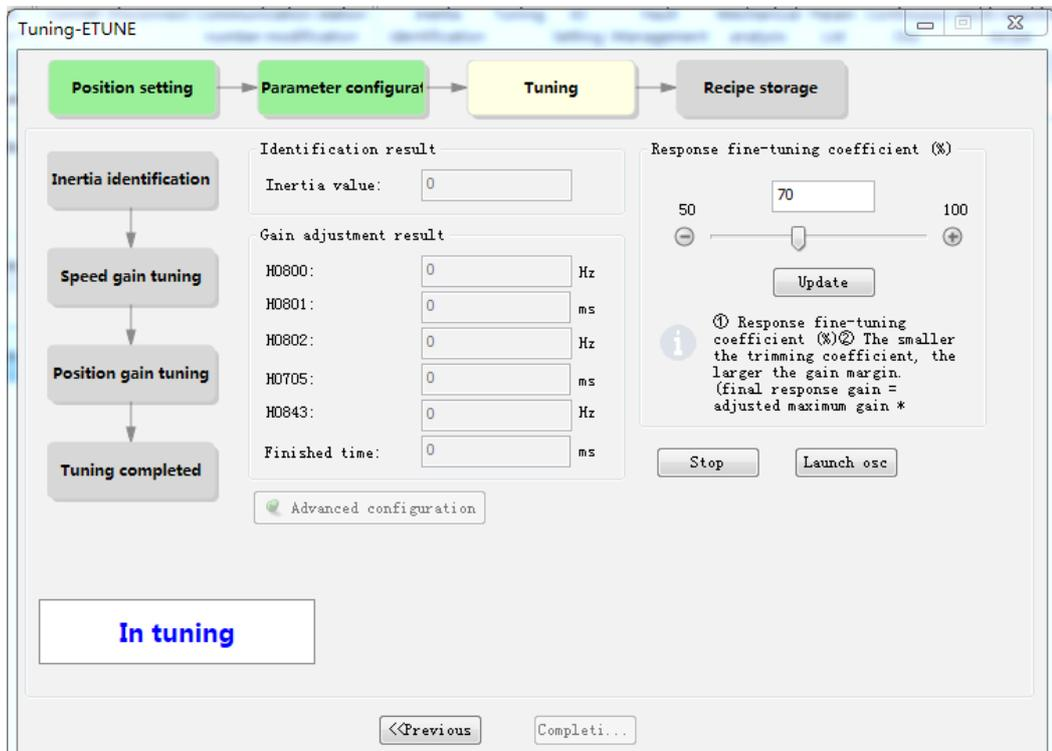
6) During gain tuning, if you modify the **Response fine-tuning coefficient** and click **Update**, gain tuning will be continued based on the fine-tuning coefficient entered. After gain tuning is done, you can click **DONE** to save the parameters to EEPROM and export parameters as a recipe file.
