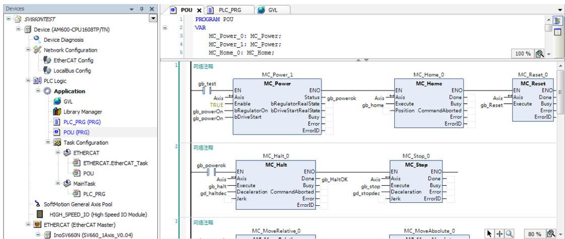
To implement directional motion through the logic program, call variables through different POU's and set the variables as global variables.
