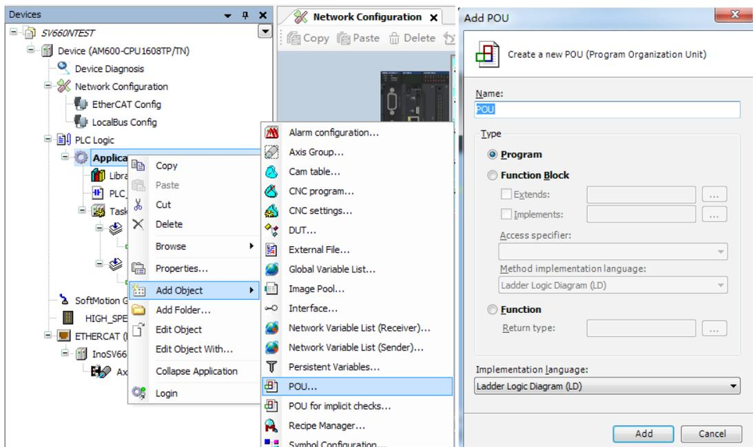
Implement the basic functions such as homing and positioning through adding the function blocks.
