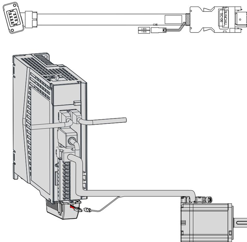
Figure 3-17 Wiring example of absolute encoder signals<sup>[1]</sup>
