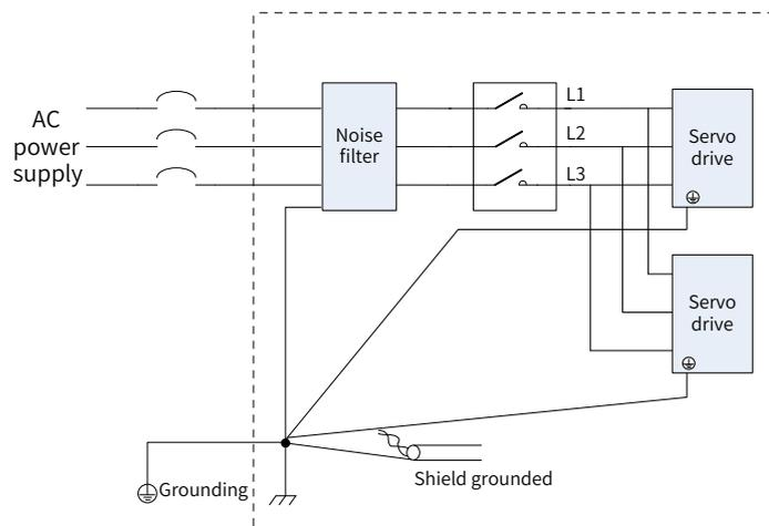
Figure 3-30 Grounding cable of the noise filter
