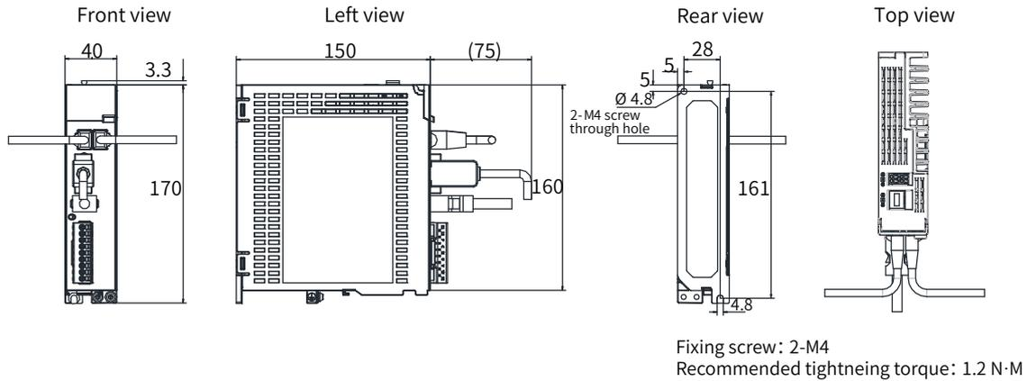
Figure 2-1 Outline dimensions of size A (unit: mm)
