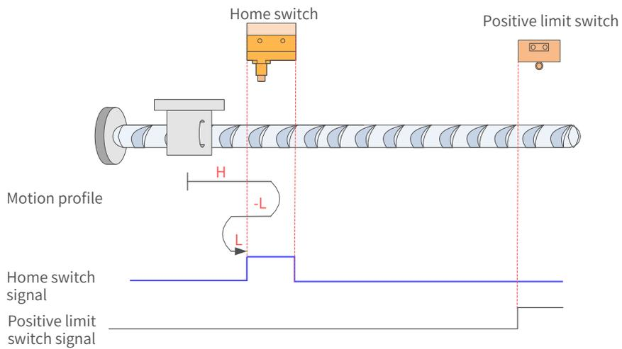
Figure 7-63 HW signal inactive at start, not hitting the positive limit switch
