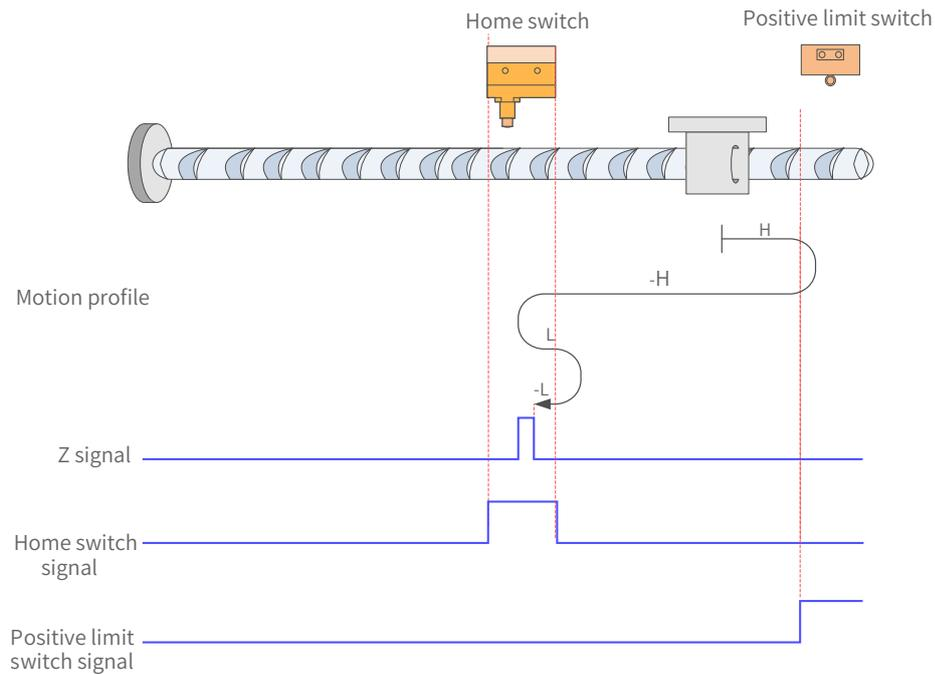
Figure 7-31 HW signal inactive at start, hitting the positive limit switch
