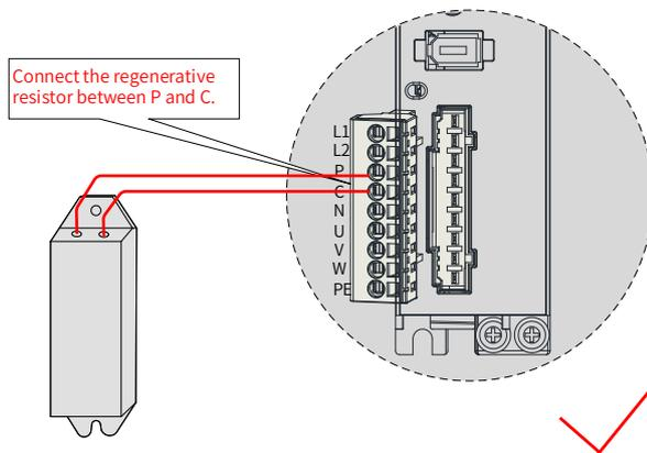
Figure 5-8 Connection of an external regenerative resistor
