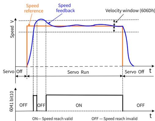
If the difference value between the speed reference and speed feedback is within  $\pm 606D$  and such status persists for the time defined by 606E, the speed is reached, and bit10 (Target reached) of 6041h is set to 1.
