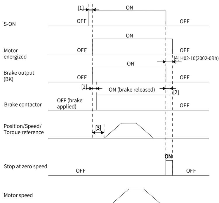
Figure 5-4 Brake time sequence for motor at a standstill
