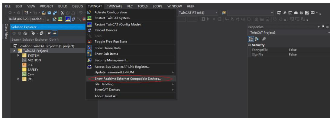
Open **Show Real Time Ethernet Compatible Devices...** in the menu shown in the preceding figure to display the following dialog box. Select local connection under **Incompatible devices**, and click **Install**. After installation is done, the network adapter installed will be displayed under **Installed and ready to use devices(realtime capable)**.
