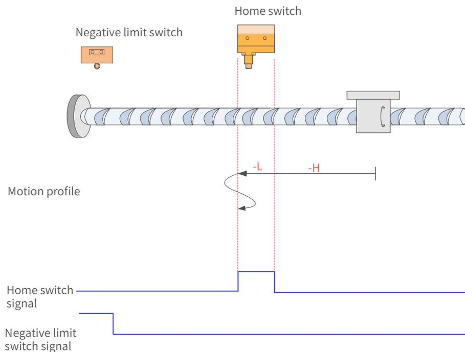
Figure 7-81 HW signal inactive at start, not hitting the negative limit switch
