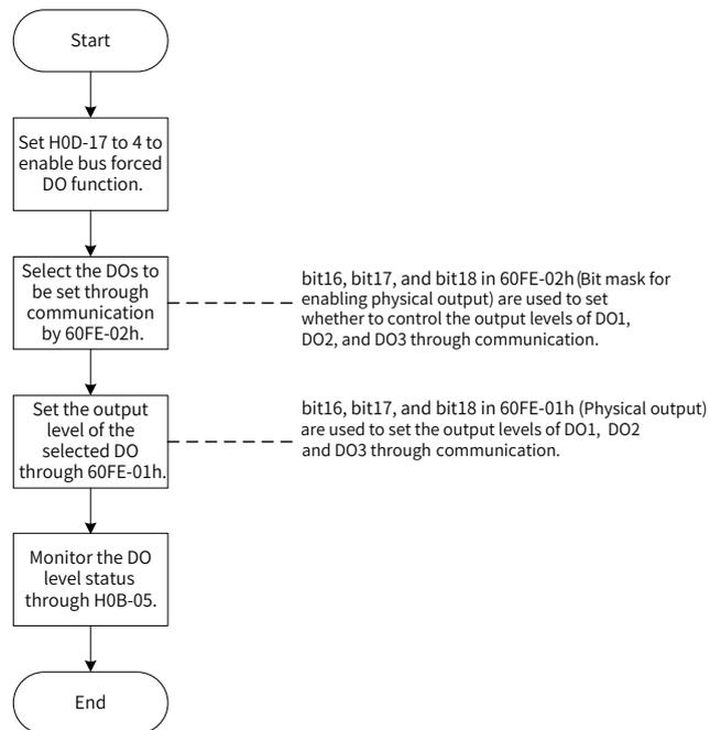
Figure 4-15 Procedure for setting forced DO through EtherCAT
