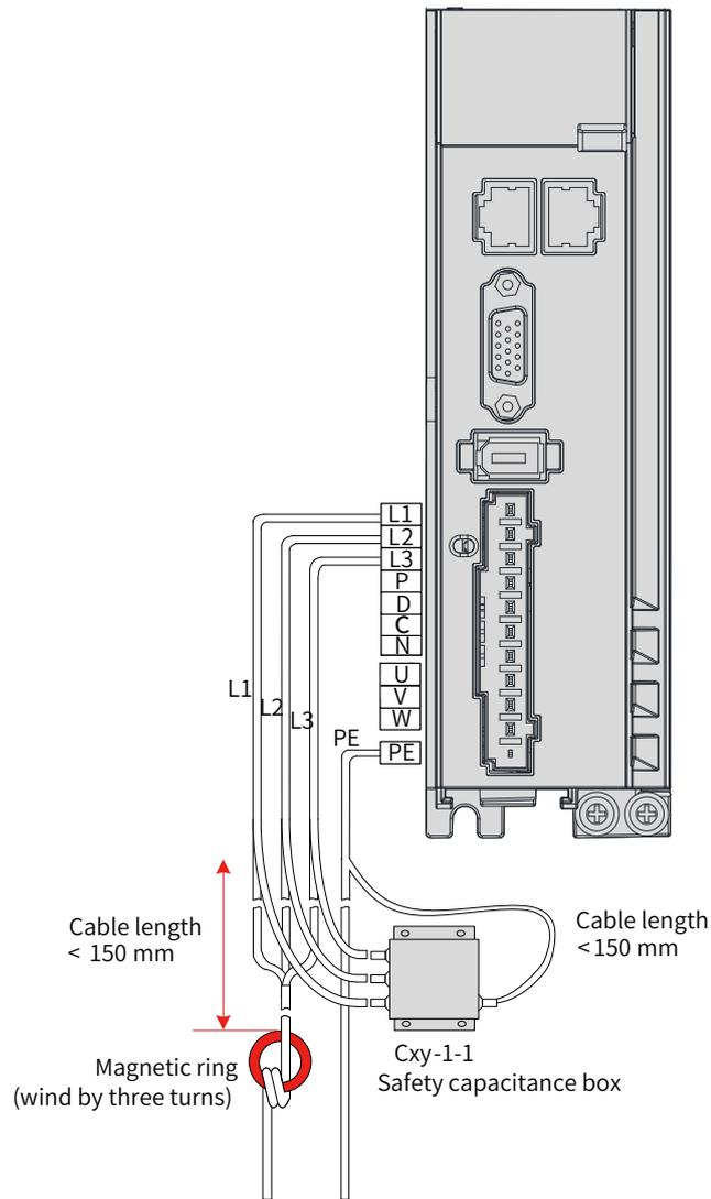
Figure 12-6 Installation of the capacitance box and the magnetic ring
