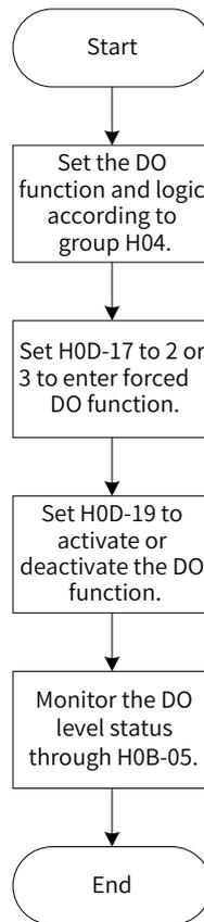
Figure 4-11 Procedure for setting forced DO function
