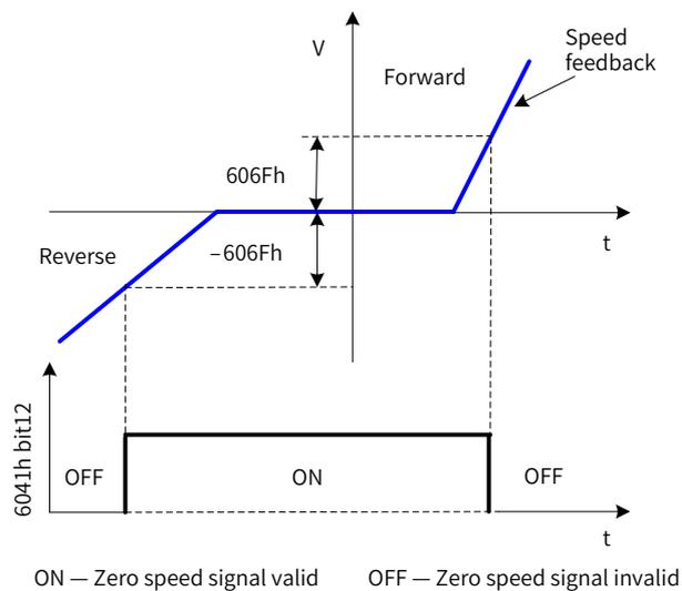
When the speed feedback is within  $\pm 606F$  and such status persists for the time defined by 6070, bit12 of 6041 is set to 1, indicating the motor speed is 0.
