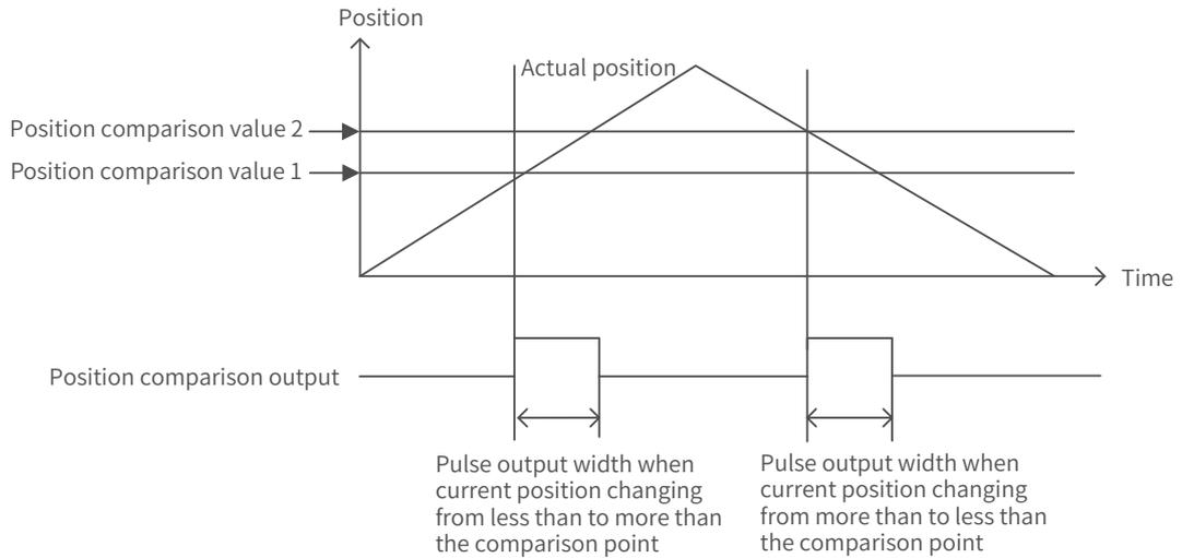
When the attribute of the comparison point is set to 1 (Output DO active signal if current position changes from "less than" to "more than" the comparison point), the DO outputs the position comparison signal when the axis position changes from "less than" to "more than" the comparison point position.
