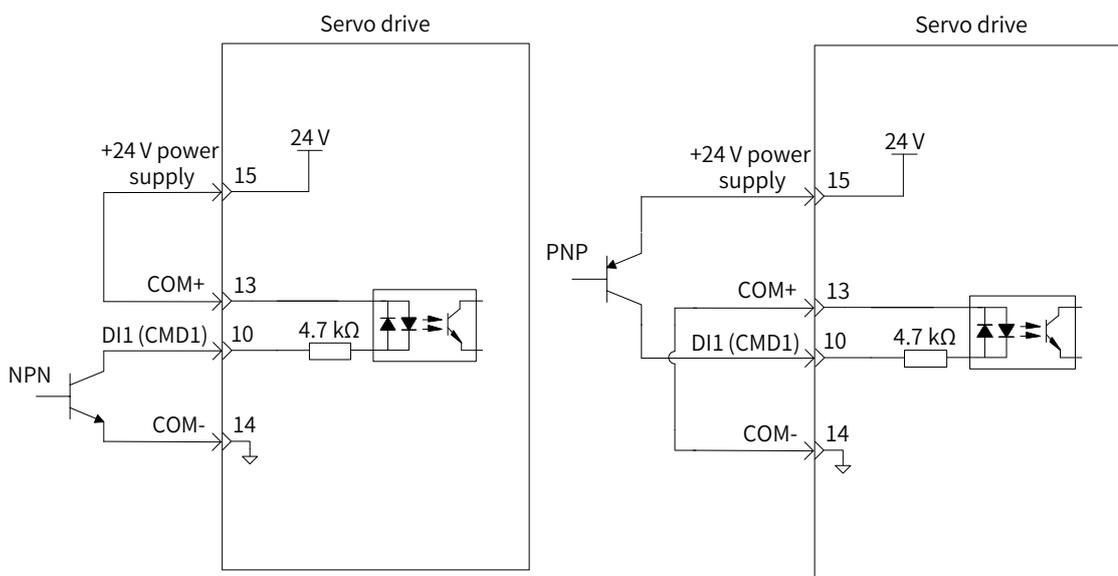
■ When using an external power supply
