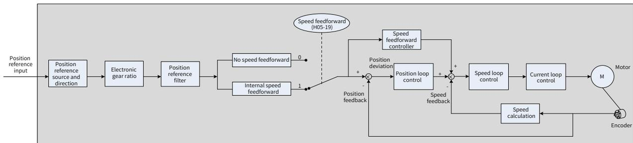
Figure 6-8 Operating process for speed feedforward control
