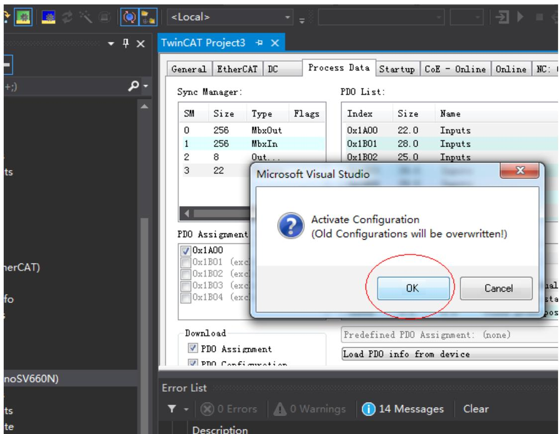
c) After clicking **OK**, the device enters OP status as shown in the **Online** interface. The 3rd LED on the keypad displays the value 8, and the keypad displays \_88RY.
