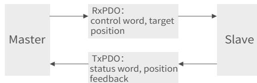
The SV660N servo drive allows users to assign the PDO list and define the PDO mapping object.
