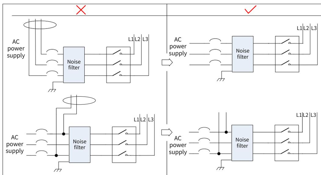
Figure 3-27 Separate routing of input and output cables
