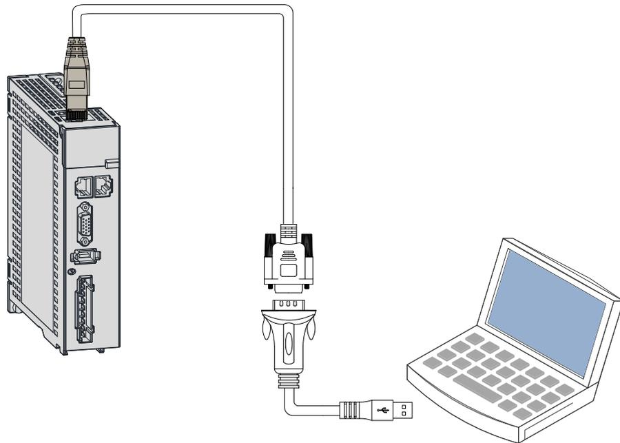
Figure 3-25 Serial-to-USB conversion
