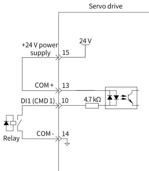
■ When using an external power supply
