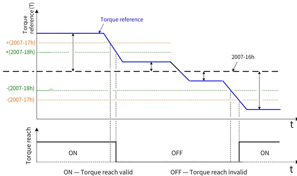
If the absolute difference value between the torque reference and 2007-16h (Base value for torque reached) is larger than 2007-17h (Threshold of valid torque reach), the torque reached signal is valid. Otherwise, the original status applies.
