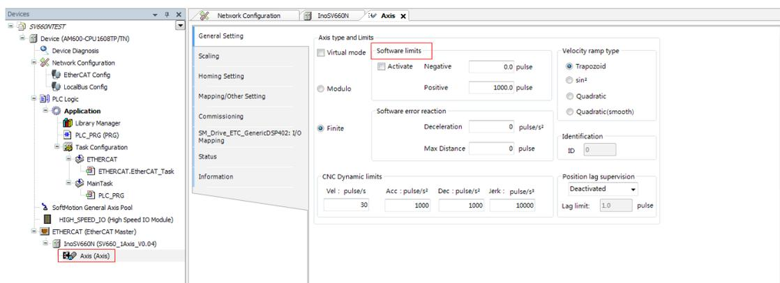
Select **16#800000** for the 23-bit encoder and **16#100000** for the 20-bit encoder during unit conversion. In Case 1, the single-turn stroke is set to 60 mm, and 1 mm/s equals to 1 RPM of the motor.
