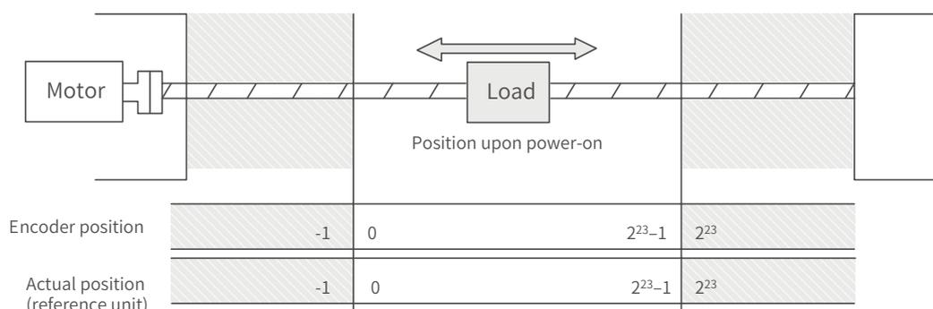
When the gear ratio is 1:1, and 607Ch is set to 10000, the position range is as shown in the following diagram.
