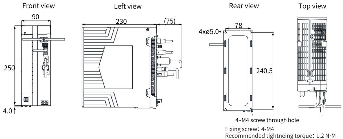
Figure 2-5 Outline dimensions of size E (unit: mm)
