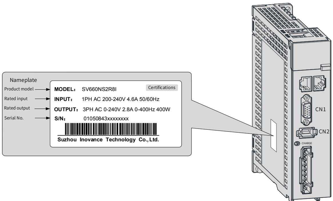
Figure 1-1 Nameplate and model number
