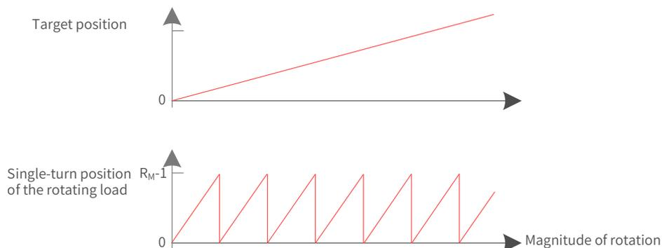
The variation law of the target position and the single-turn position of the rotating load during reverse running is shown as follows.
