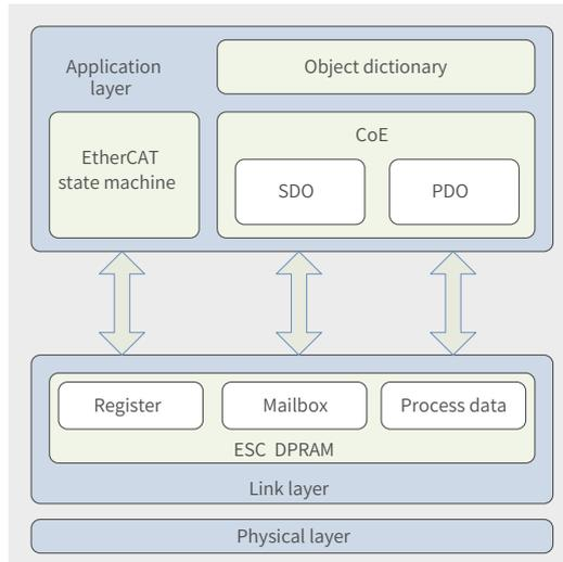
Figure 9-2 EtherCAT communication structure with CANopen application layer
