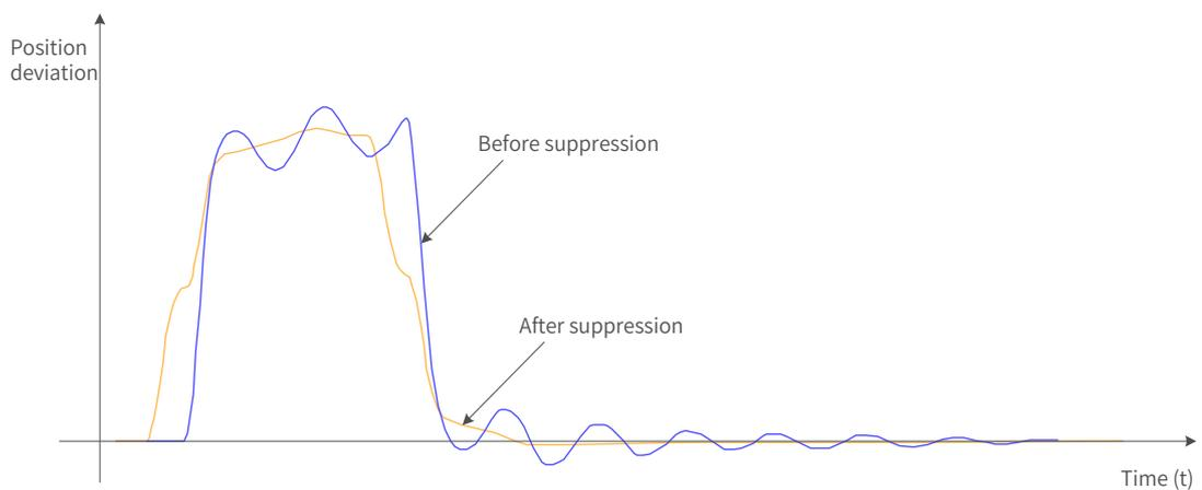
Figure 6-16 Effect of low-frequency resonance suppression
