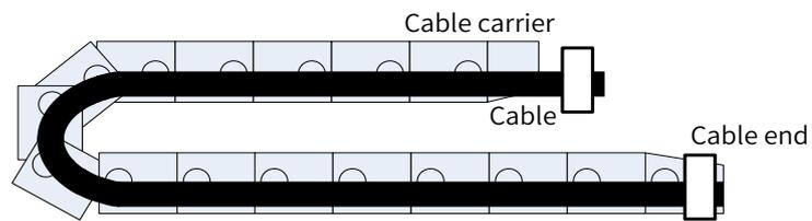
Figure 3-31 Cable carrier
