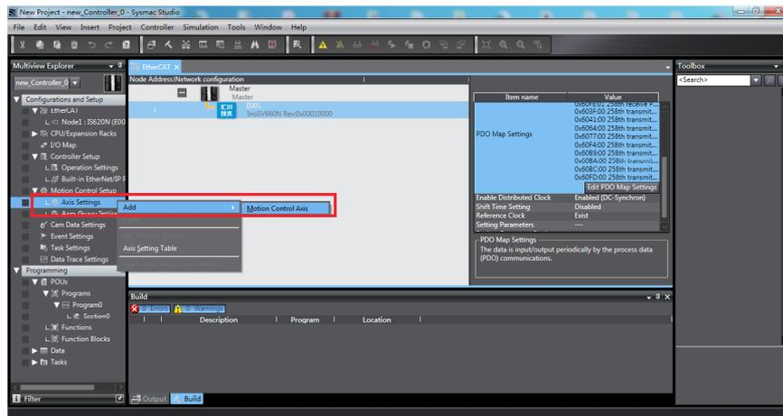
**MC\_Axis000** can be renamed through a simple click. For example, if it is named as Rewind axis, the axis variable Rewind axis used in the NX program represents control on this SV660N servo axis.
