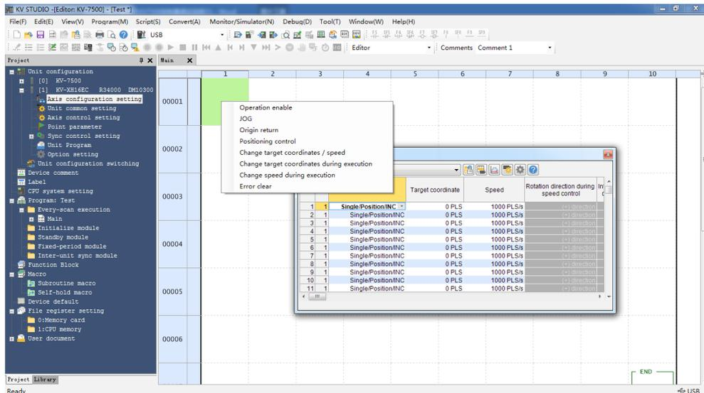
Select the function needed, such as **Operation enable**, click it to generate a DEMO program automatically. Then designate the part in red as the relay needed. After these actions are done, this function is done compiling.
