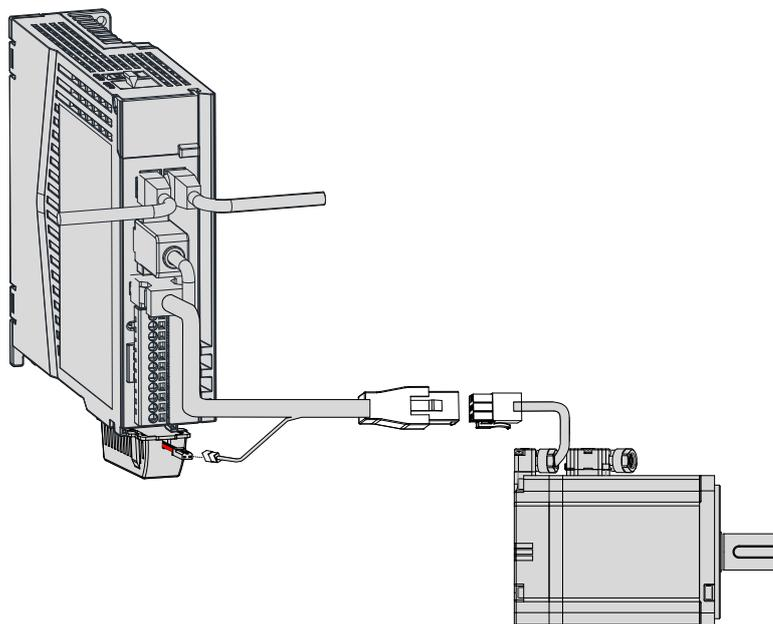
Lead wires of the battery box:
