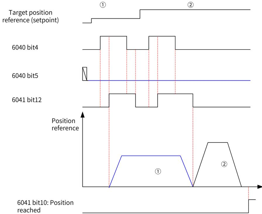
Note: To modify the target position reference (setpoint), the new target position bit (bit4) has to be sent again.
