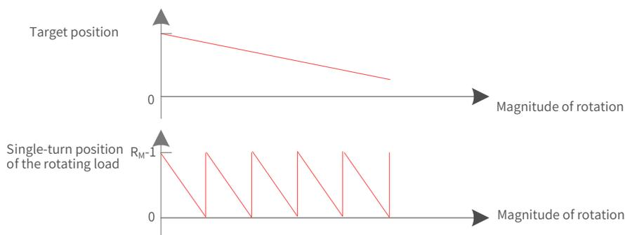
When the motor works in the absolute rotation mode and the servo drive operates in the HM mode, the setting range of the home offset is 0 to  $(R_M-1)$ . If the home offset is set to a value outside this range, the servo drive reports EE09.1 (Home setting error).
