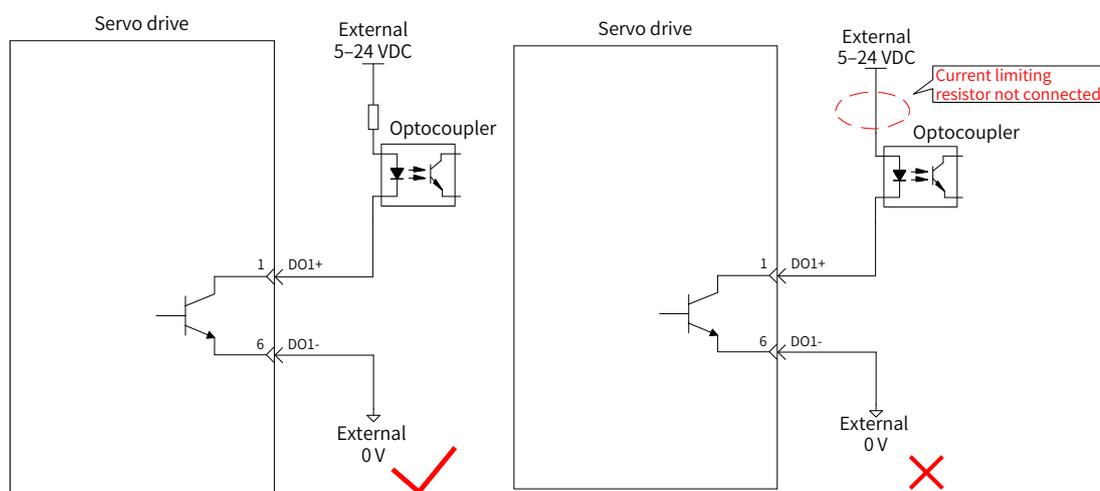
The maximum allowable voltage and current of the optocoupler output circuit inside the servo drive are as follows:
