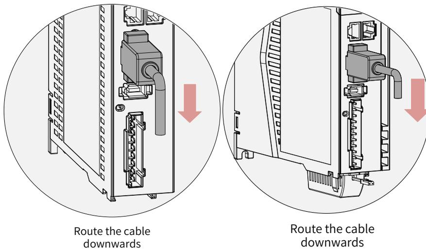
Figure 2-7 Routing direction
