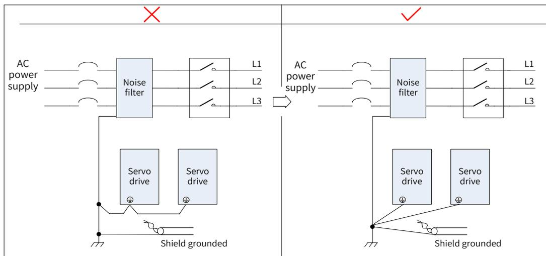
Figure 3-29 Single-point grounding
