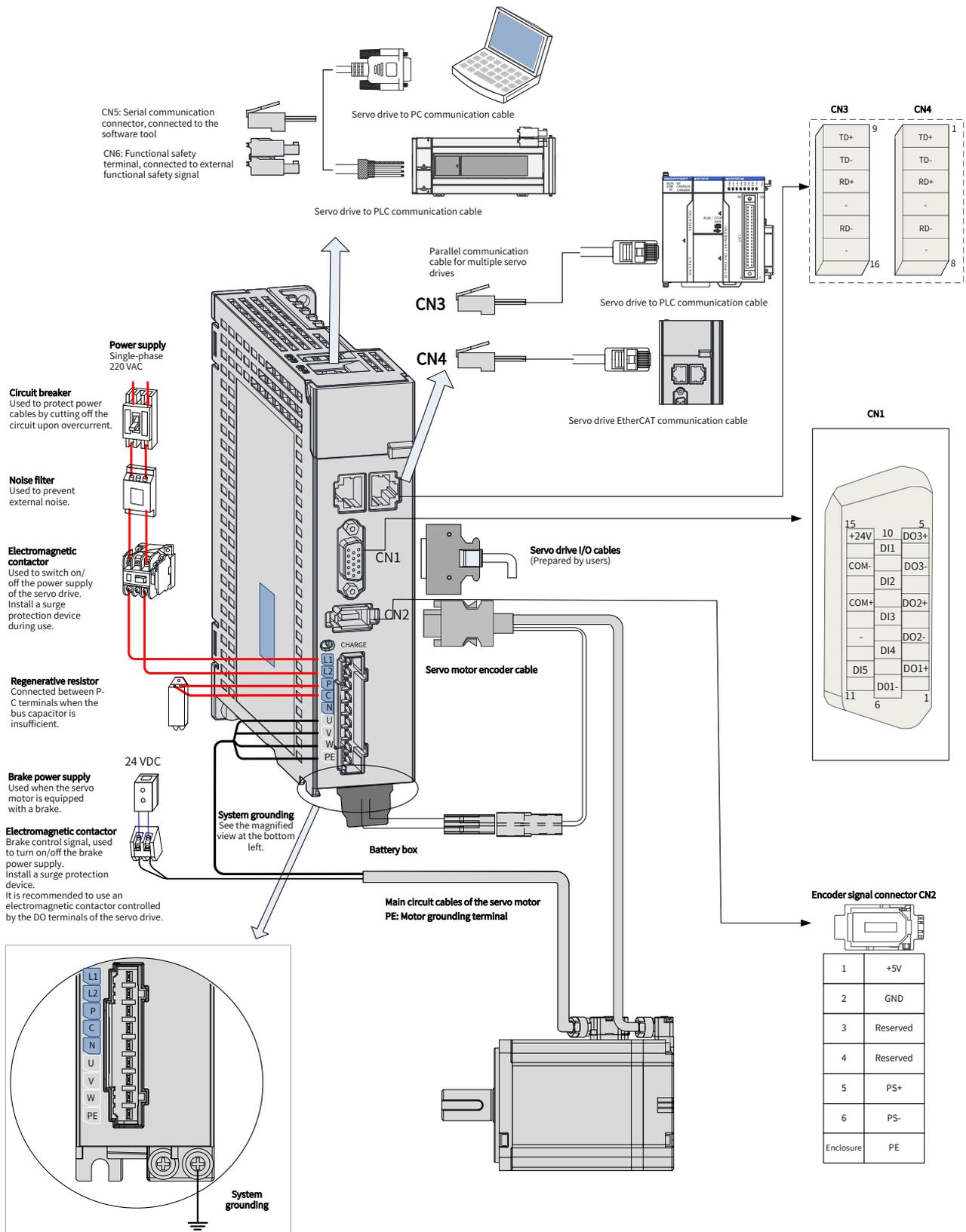
Figure 1-13 Wiring of single-phase 220 V systems
