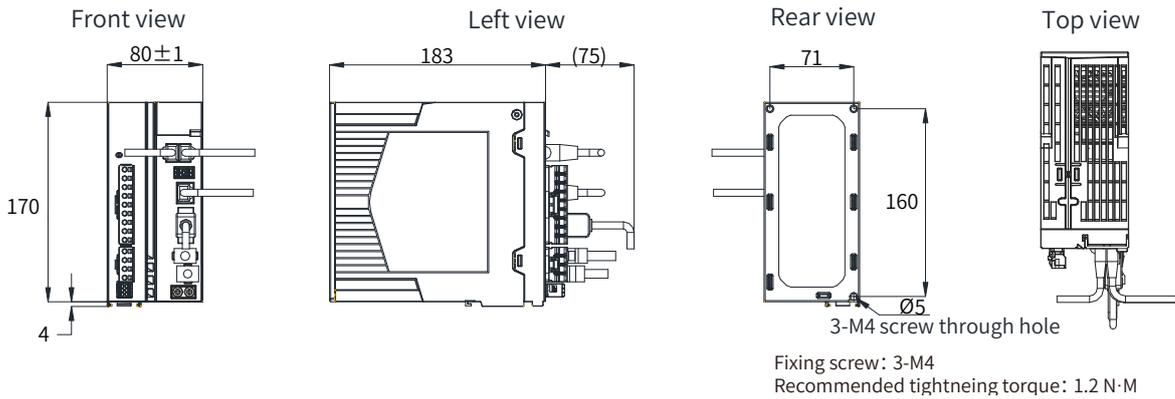
Figure 2-4 Outline dimensions of size D (unit: mm)
