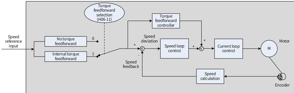
Figure 6-9 Operating process for torque feedforward control
