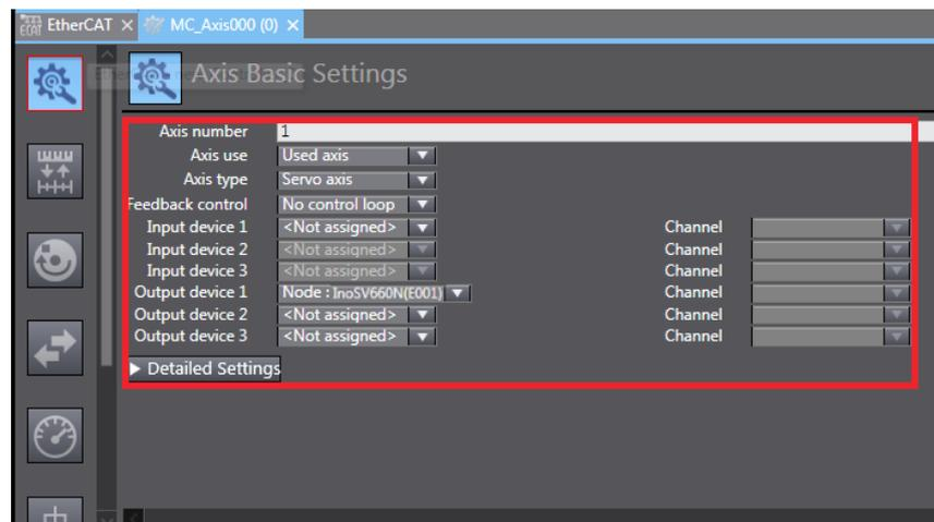
**Axis number:** Represents the Ethernet communication station No. of the servo drive, which is also the value of H0E-21.
