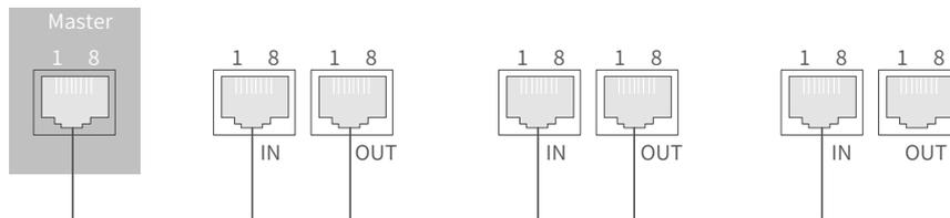
■ Redundancy ring connection
