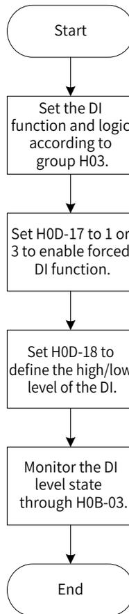
Figure 4-8 Procedure for setting forced DI function
