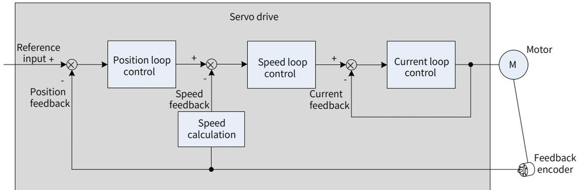
Figure 7-1 Structure of a basic servo system
