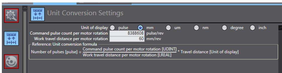
Select **Unit of display** based on the actual running unit when setting the gear ratio. All the position-type parameters in the host controller will be displayed in this unit.
