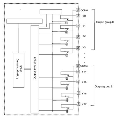
The following figure shows the internal equivalent circuit of mixed output of transistors and relays. Output terminals are divided into several groups, with each group electrically isolated. The output contacts of different groups are connected to different power circuits. Transistor outputs can be applied only to 24 VDC load circuits.
