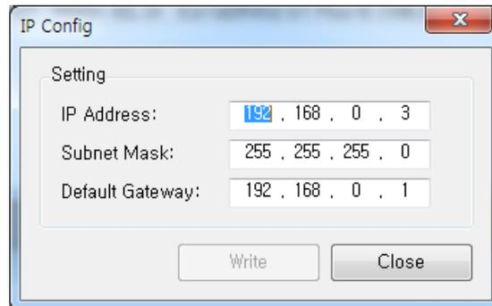
After clicking "Write" and Power reset, Configuration is applied.
