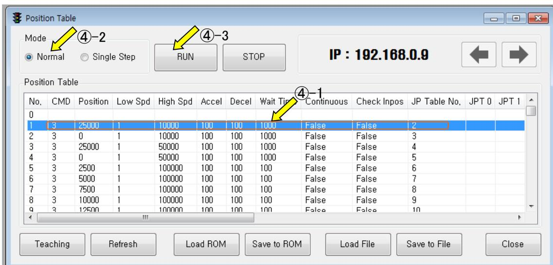
While PT No is operated in sequence, PT lines in service are changed in grey. Also, the user may monitor the operation status as described at '7.3 Position Status' and '7.4 Axis Status' through 'Motion Test' window,
