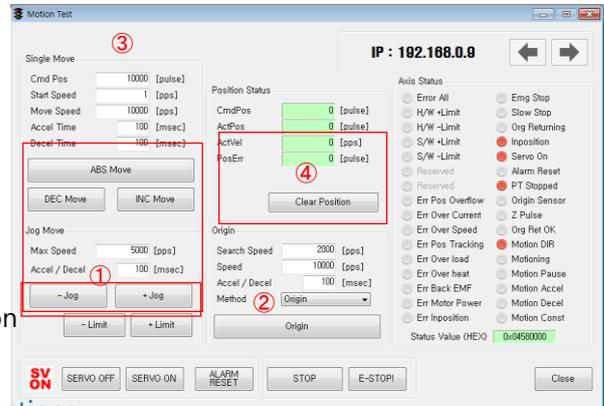
4) According to the motion of motor, the user can check its position and operation status. For more information, refer to
