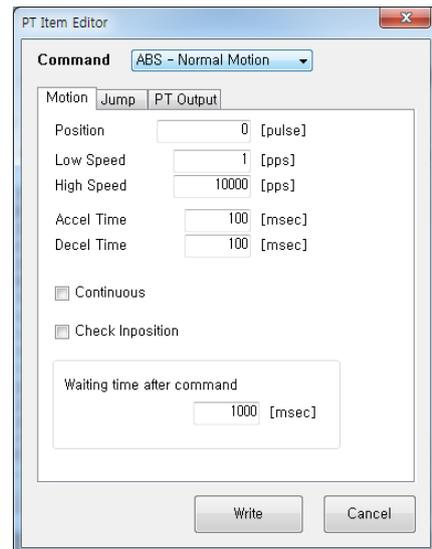
This data is saved to the RAM area. So, when power is off, data is deleted. Click 'Save to ROM' button, and save the data to the ROM area.
