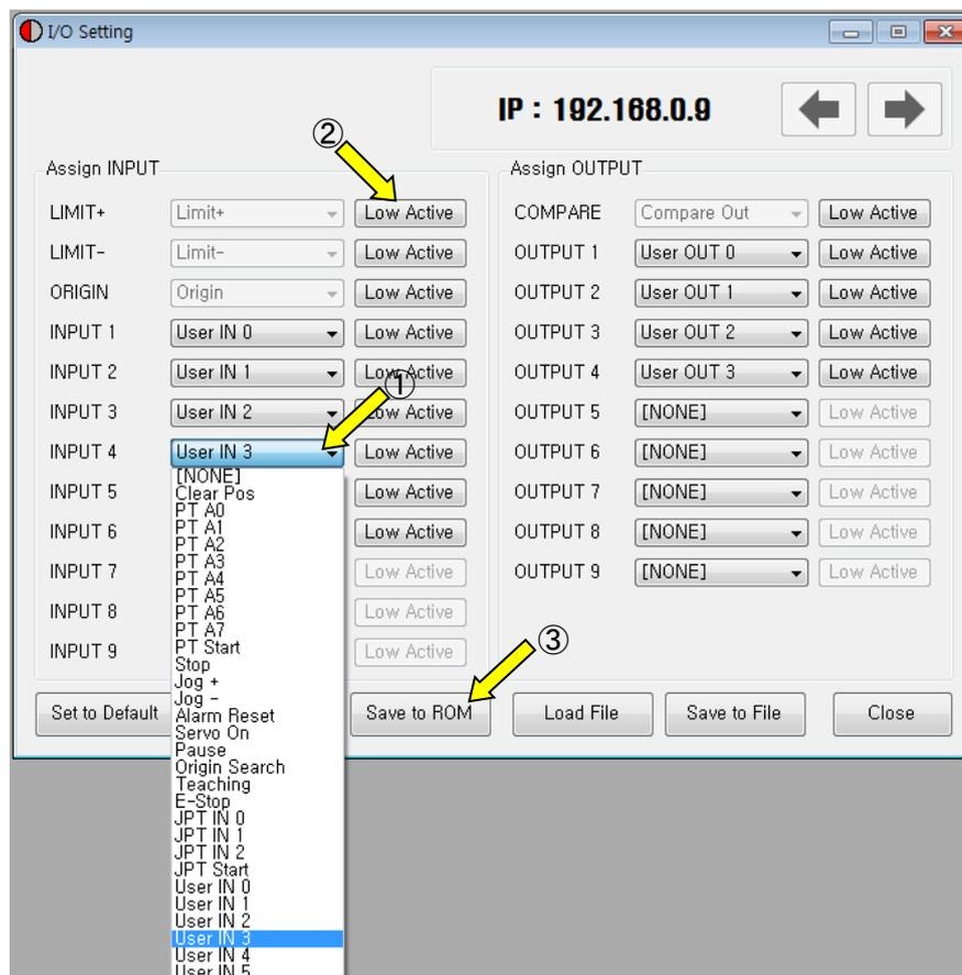
The assignment method of input and output is same and using as following
