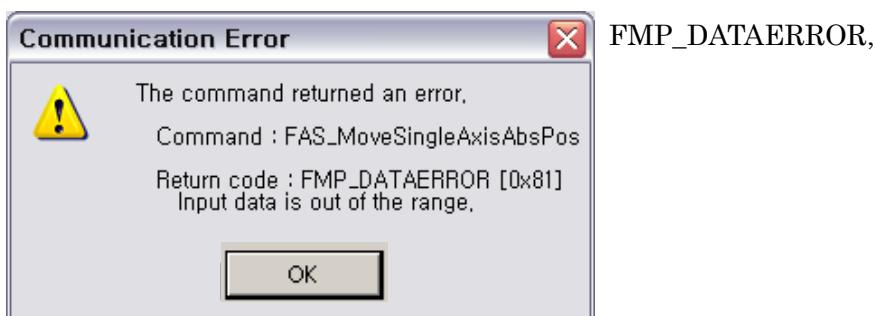
The value of the sent data is out of the proper range of the drive.
