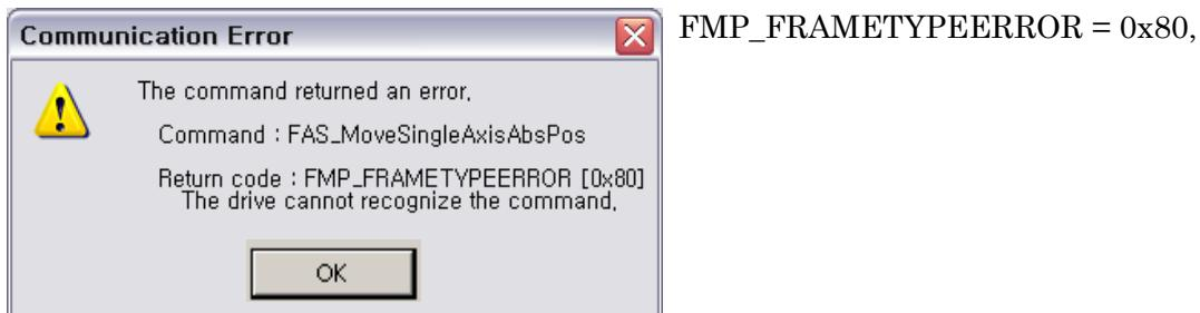
Drive does not recognize the command or wrong command is sent.
