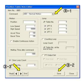
This data is saved in the RAM area. So, when power is off, data is deleted. Click 'Save to ROM' button, and save the data to the ROM area.
