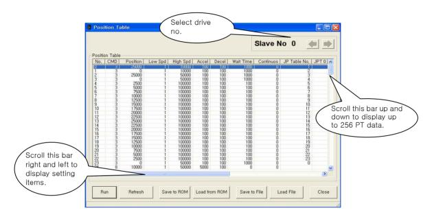
Position table data can be changed at any time. The position table can sa ve up to 256 step data. If the position table is used to the program area, it may be used for all point numbers without restriction. That is, it is possible to start at a random point number and jump to other point number.
