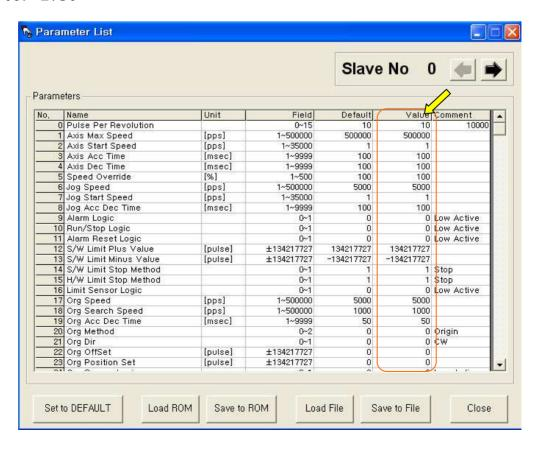
The user can set and save parameter values related to motion control by each drive module. 'Value' column displays the value applied to current motion control and can be edited.
