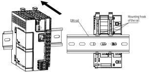
Make sure the DIN rail mounting hook of the module is locked. The locked and unlocked states of the mounting hook are shown below.
