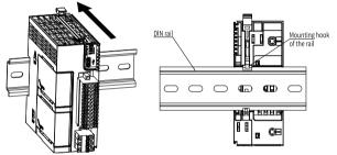
Make sure the DIN rail mounting hook of the master is locked. The locked and unlocked states of the mounting hook are shown below.
