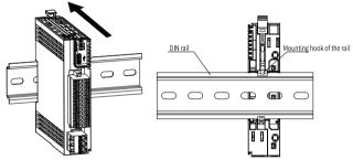
Make sure the DIN rail mounting hook of the controller is locked. The locked and unlocked states of the mounting hook are shown below.
