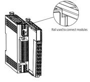
Install an DIN rail end plate to both sides of the master or module. To mount the end plate, hook the bottom of it to the bottom of the DIN rail, rotate the end plate to hook the top of it to the top of the DIN rail, and then tighten the screw to lock the end plate in place, as shown below.
