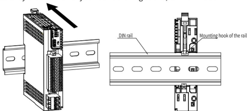
2. Make sure the DIN rail mounting hook of the controller is locked. The locked and unlocked states of the mounting hook are shown below.
