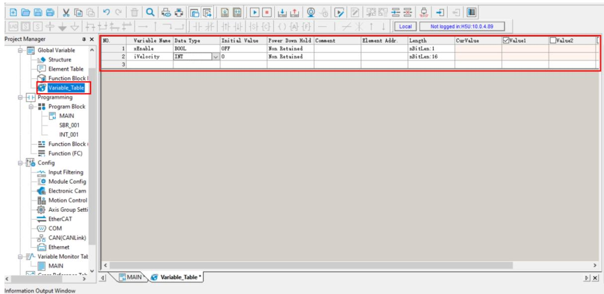
When write directly in the program editor, and then press the ENTER key or click the area outside the basic block of the program the editor interprets that it is a name of a variable and opens the dialog box that allows to declare the variable that will be added to the general table of variables.
