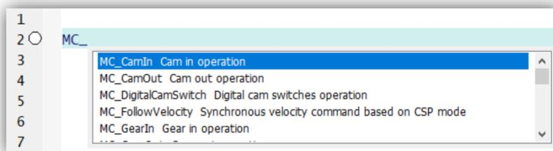
You can select the desired command and press ENTER for the editor to finish typing the full name of the command.
