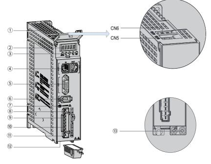
Figure 2-1 Components of servo drives in size A (SV660FS1R6I, SV660FS2R8I)
