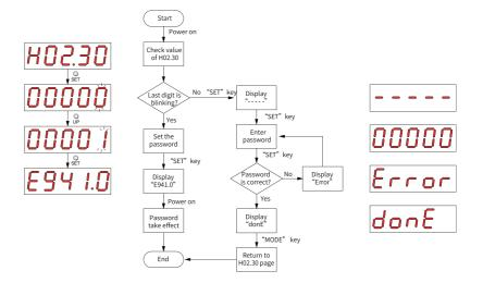
Figure 5-15 Procedure for setting the user password
