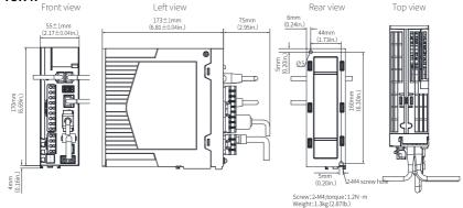
Figure 3-7 Dimension drawing of servo drives in size C
