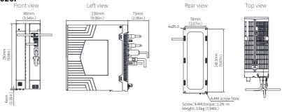
Figure 3-9 Dimension drawing of servo drives in size E
