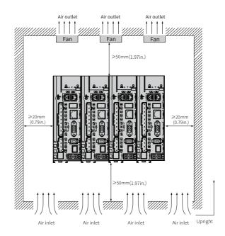
Figure 3-4 Zero-clearance installation
