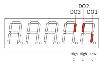
Figure 5-14 Display of H0b.05 when DO signals are controlled by the bus
