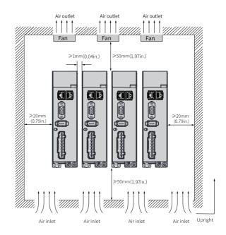
Figure 3-3 Clearance for compact installation
