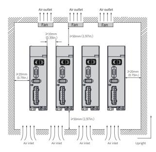
Figure 3-2 Clearance for side-by-side installation
