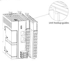
Mount an end plate on a side of the PLC or expansion module. To mount the end plate, hook the bottom of it to the bottom of the DIN rail, rotate the end plate to hook
