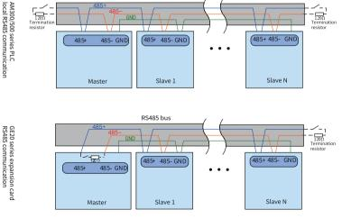
To avoid interference, do not bundle the cable together with an AC power cable or high voltage cable.
