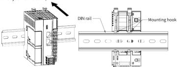
Make sure the DIN rail mounting hook of the PLC is locked. The locked and unlocked states of the mounting hook are shown below.
