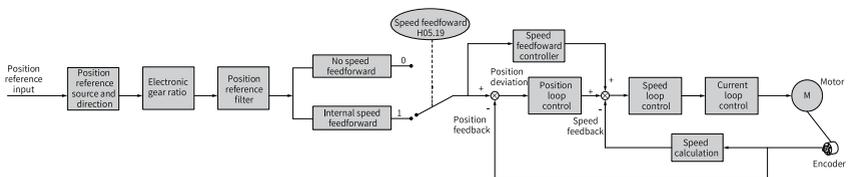
Figure 3-10 Operating procedure for speed feedforward control
