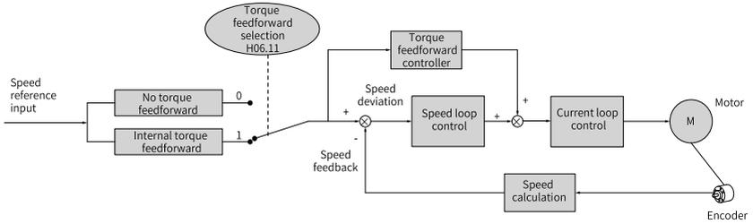
Figure 3-12 Operating procedures for torque feedforward control
