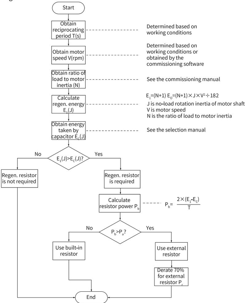
Figure 2-8 Flowchart for selecting the regenerative resistor
