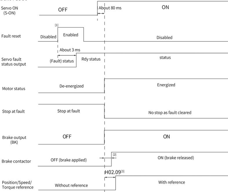
Figure 2-22 Sequence for fault reset
