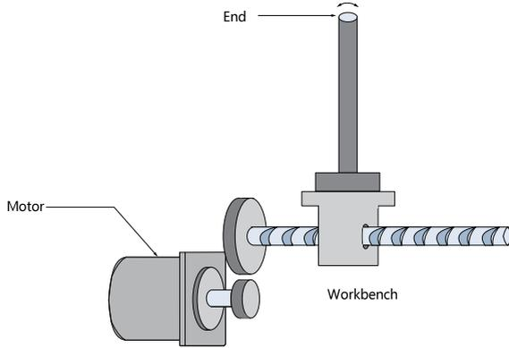
Figure 3-17 Low-frequency vibration at the mechanical end
