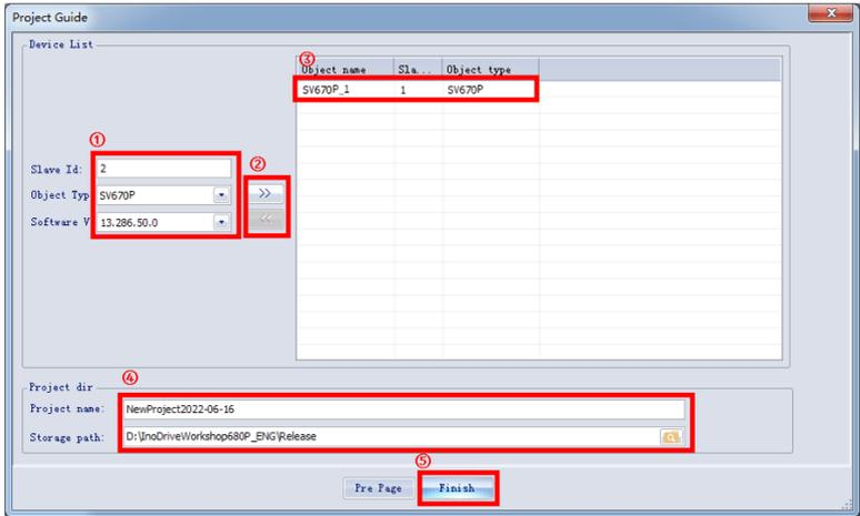
Figure 1-19 **Project Guide** interface for offline device
