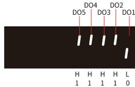
Figure 1-14 Display of H0b.05 when DO signals are controlled by the bus
