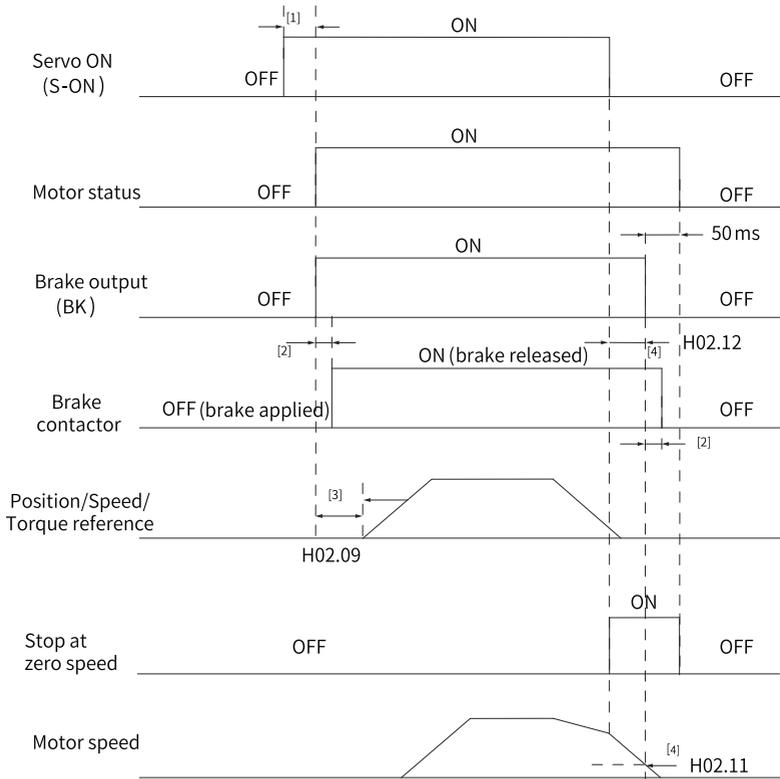
Figure 2-6 Brake sequence for a rotating motor
