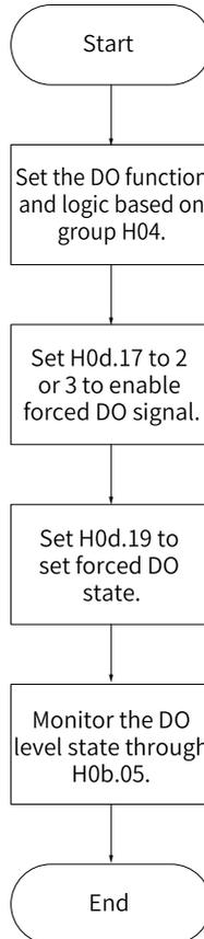
Figure 1-9 Procedure for setting forced DO function
