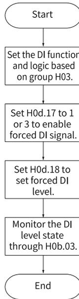
Figure 1-6 Procedure for setting forced DI function
