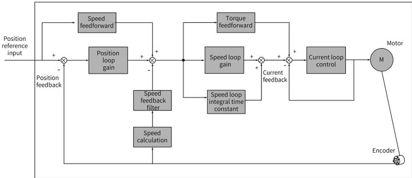
Figure 3-7 Basic control for manual gain tuning
