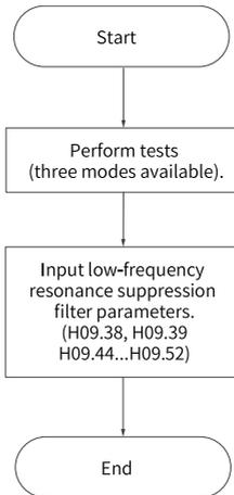
Figure 3-18 Procedure for setting low-frequency resonance suppression filter
