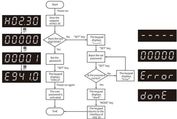
Figure 1-15 Procedure for setting the user password
