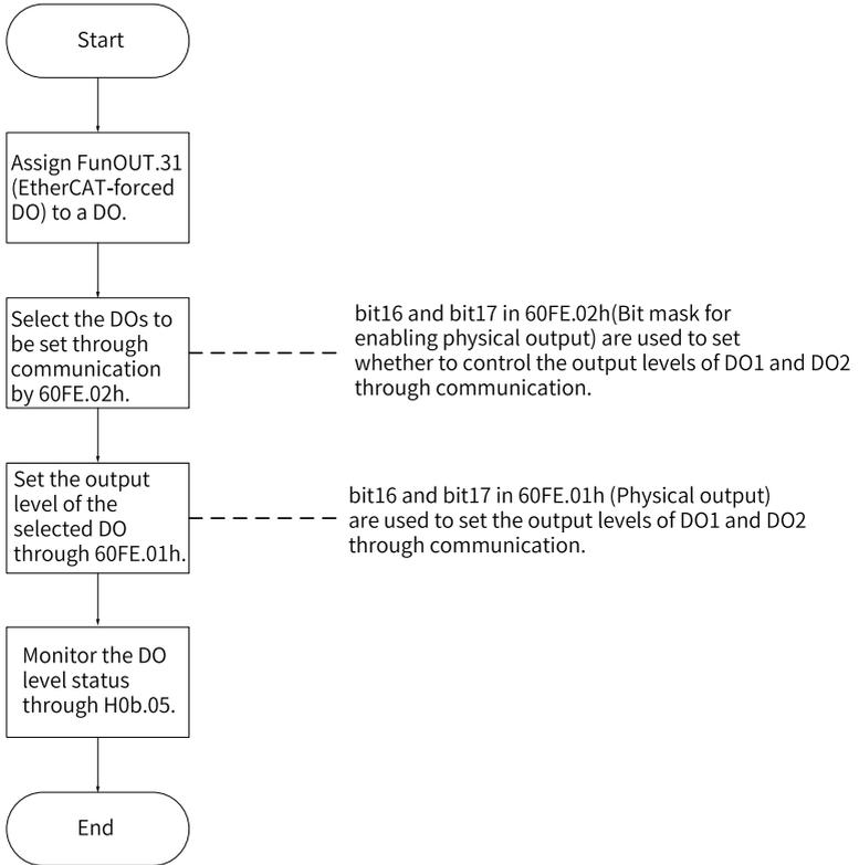
Figure 1-13 Procedure for setting bus control forced DO function
