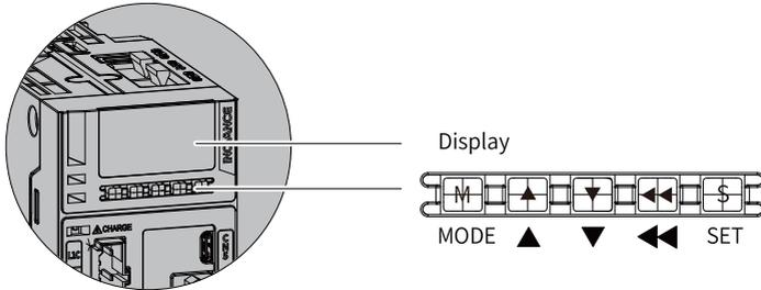
Figure 1-1 Magnified view of the keypad
