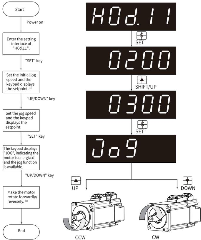
Figure 2-2 Procedure for setting the jog function
