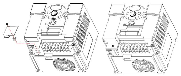
For models SINUS N 0003/0005 as shown above, loosen the bolt on the connector for Comm. Option and tighten it onto the supporter on the inverter case. Before fixing the option board, bottom cover plastic part for Comm. Option should be removed using knife or driver. The same method is used as 0001/0002 installation.
