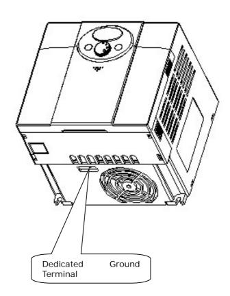
Note : Remove front and bottom cover before starting grounding.
