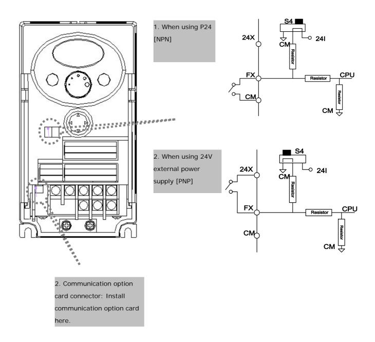
■ Note: MODBUS RTU option card is available for SINUS N. Refer to MODBUS RTU option card manual for more details.
