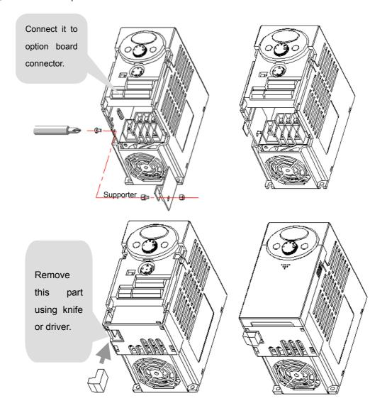
Figure 2. ModBus-RTU card installation
