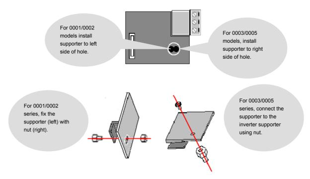
There are two holes on the option board for connection of option and inverter. Use left hole for models SINUS N 0001/0002 and right for models SINUS N 0003/0005 series.
