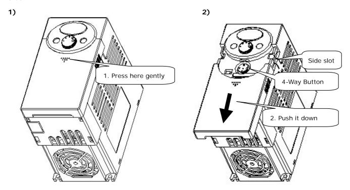
Removal for wiring: The method is the same as shown in 1. Hold both sides of the cover and lift upward to completely remove from the main body. 2. Hold both
