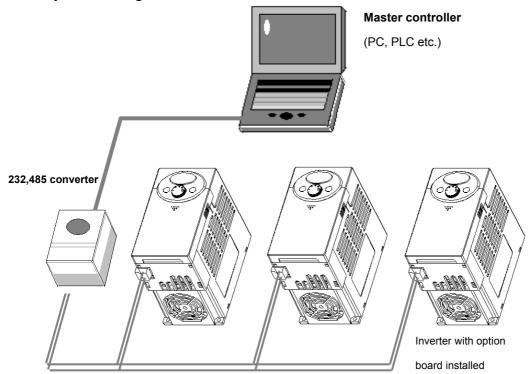
Figure 2. System configuration
