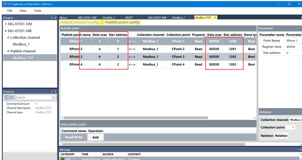
After completing the above settings, the Modbus TCP client can use the Modbus TCP protocol to access the gateway through the gateway IP address 192.168.1.254, Modbus data communication port 502, and access the collected data. This document uses Modbus Poll to simulate Modbus TCP client to collect data.
