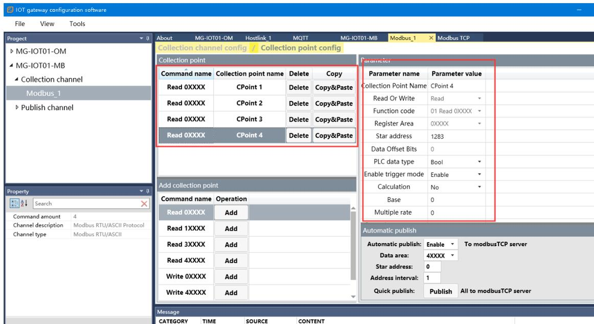
Right-click the publish channel to manually add the MQTT channel and set the configuration parameters manually. Port number: 1883, connection mode: IP address, MQTT server IP: 192.168.1.50 (local machine network card IP address, the machine simulates the MQTT server).
