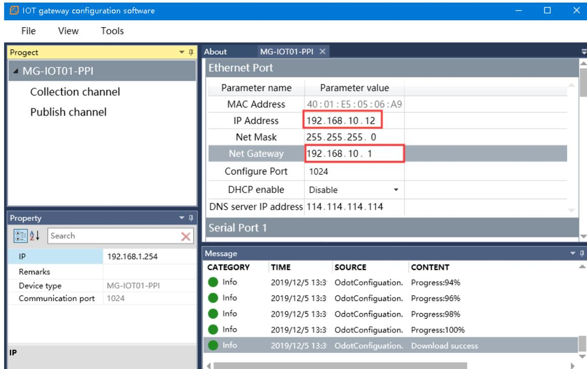
After the IP address is successfully changed, you need to change the local computer's IP address to: 192.168.10. \* Network segment.
