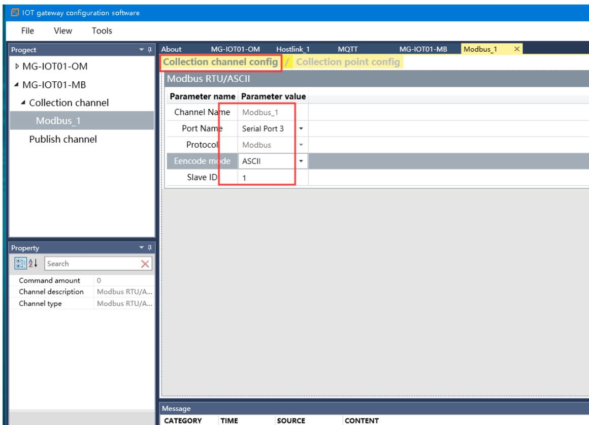
The corresponding Modbus address of Delta's PLC output coil Y is shown in the table below. Configure the collection points according to the point table. After the configuration is complete, click to publish to Zone 4.
