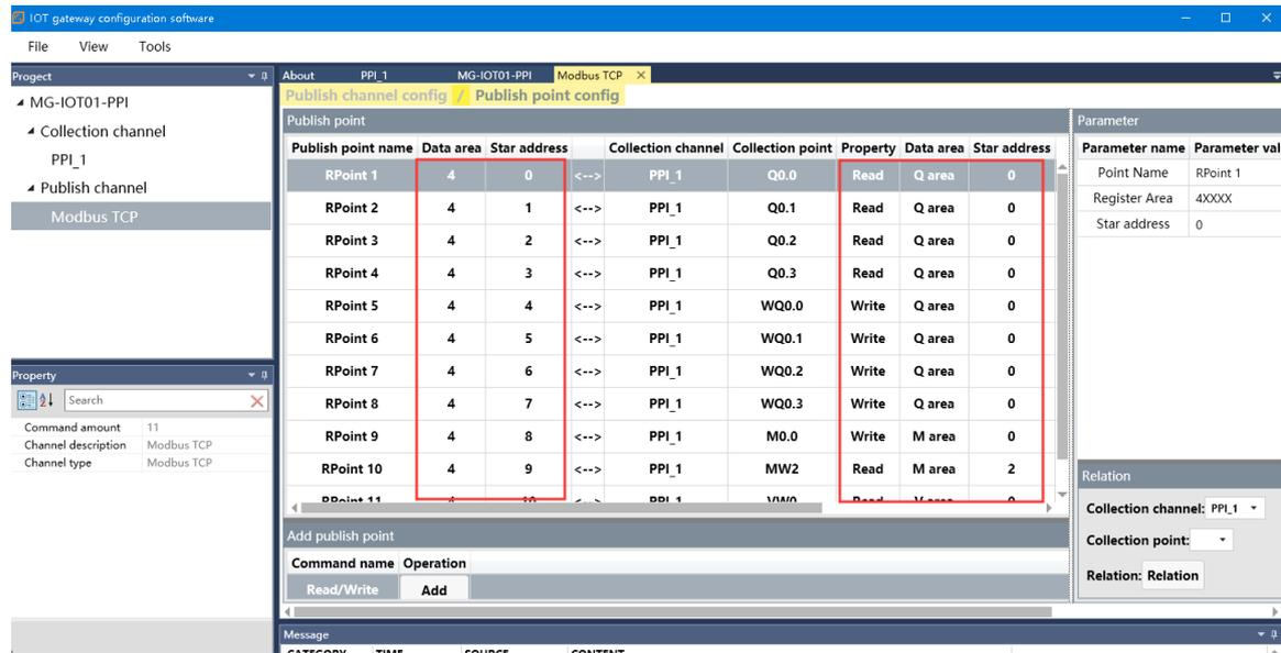
After completing the above settings, the Modbus TCP client can use the Modbus TCP protocol to access the gateway through the gateway IP address 192.168.1.254 and Modbus data communication port 502 to access the collected data. This document uses Modbus Poll to simulate Modbus TCP client to collect data.
