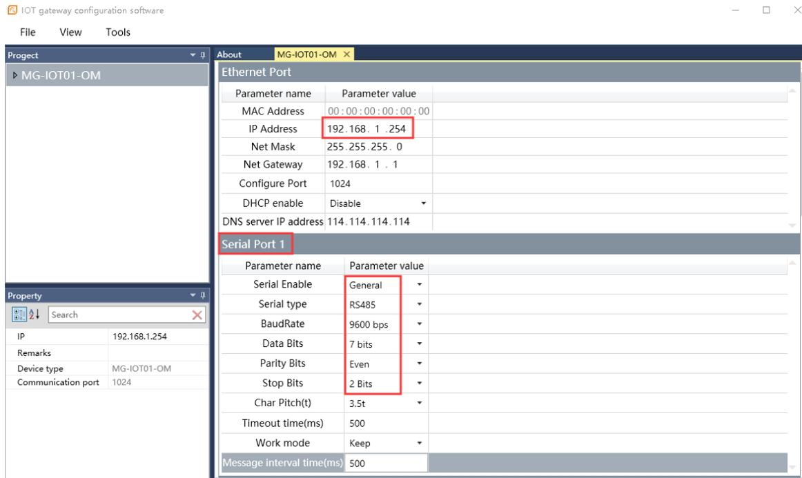
Configure the Collection channel parameters as shown below:
