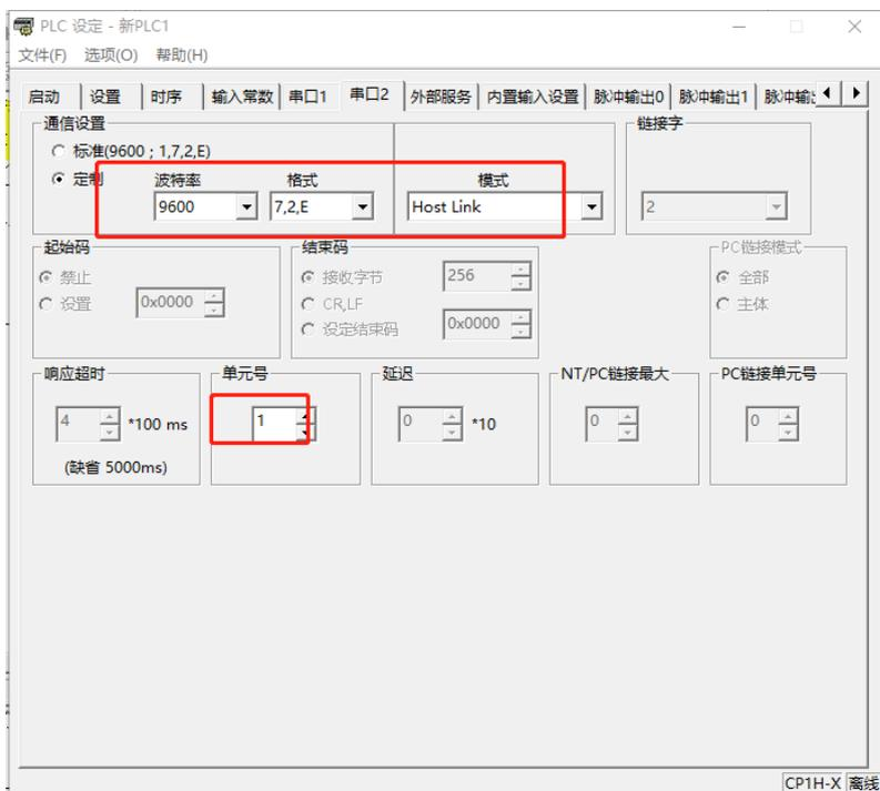
The test programming interface is as follows: After editing, save and download. Put PLC in RUN.
