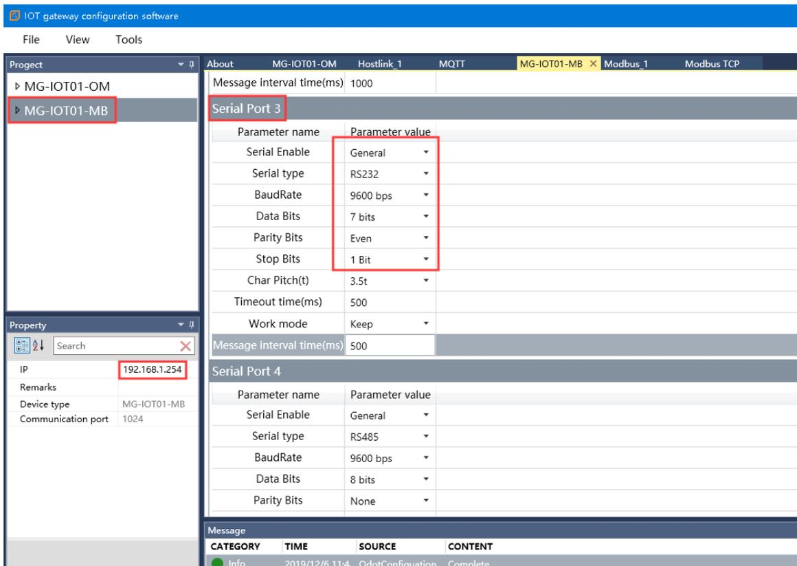
Configure the collection channel parameters as shown below:
