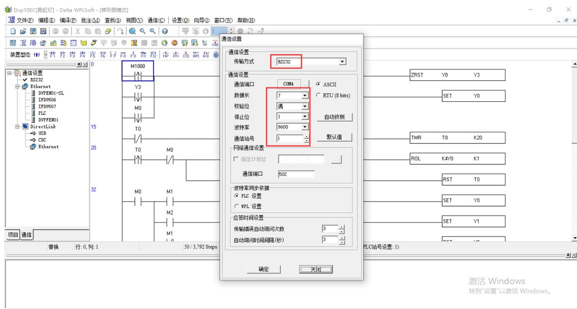
The test programming interface is as follows: After editing, save and download. Put PLC in RUN.
