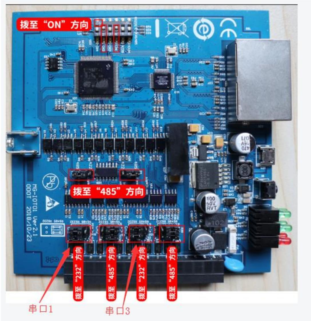
3. When the gateway device adopts the RS422 communication interface, the hardware dialing code is as follows:
