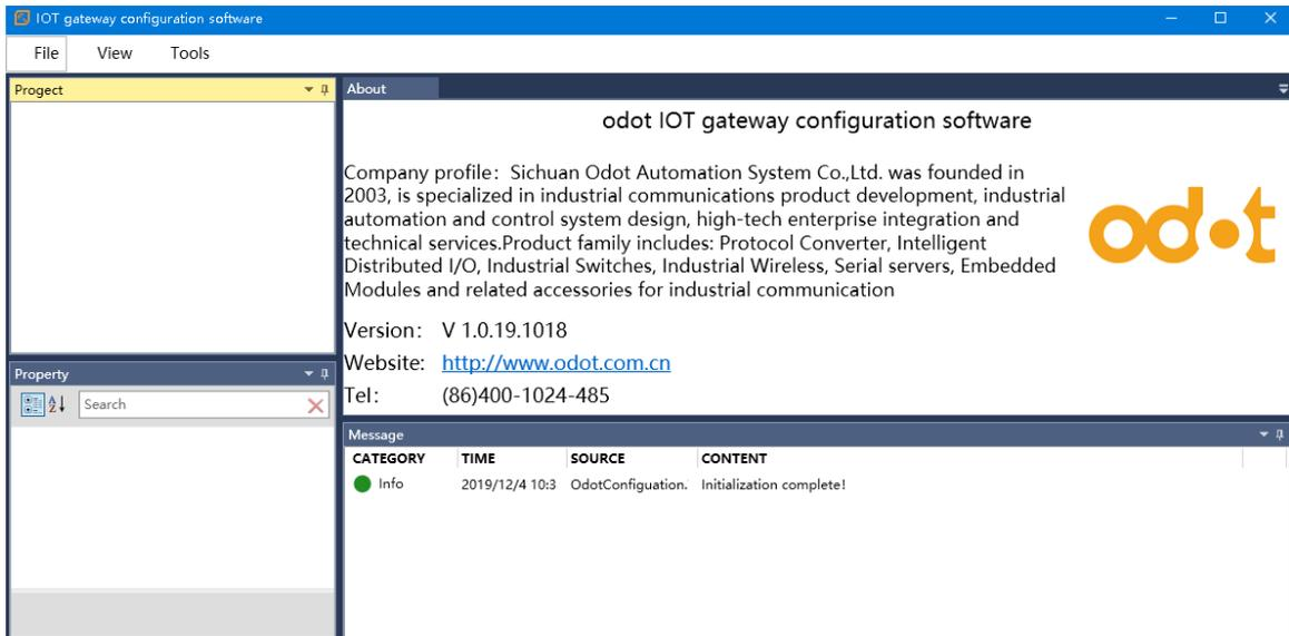
2. It consists of a Project bar, a Property bar, an Output bar, and a Configuration Information bar. Create a Project and select Configuration Information in the Project bar and configure it in the Configuration Information bar.
