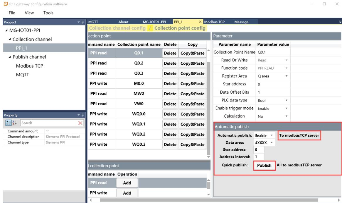
Selects the Modbus TCP channel as publish channel manually. Double-click on the right side to configure the publish channel parameters, such as Modbus port, Watchdog and other parameters.
