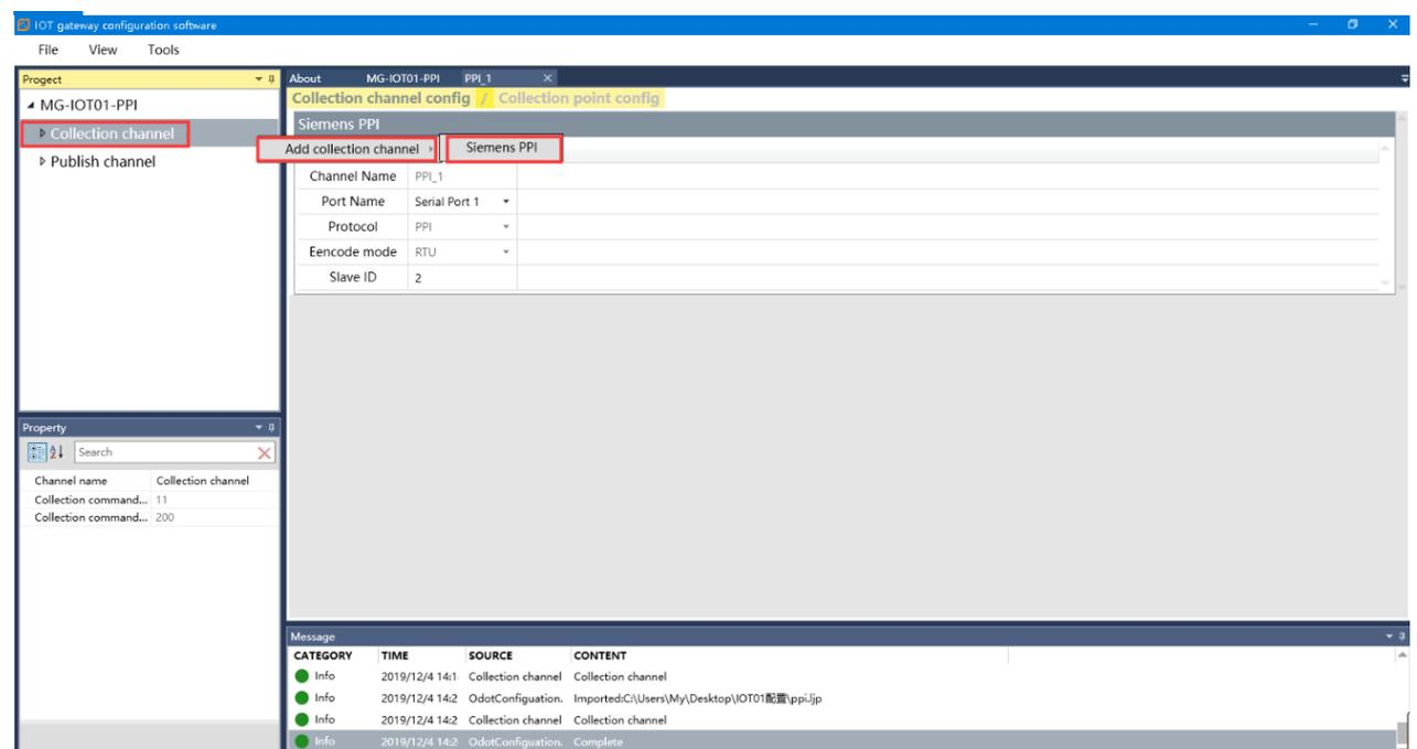
Double-click PPI\_1, and the Collection channel config window pops up on the right. In the Collection channel config window, set the serial port to confirm which serial port to collect and the Slave ID.
