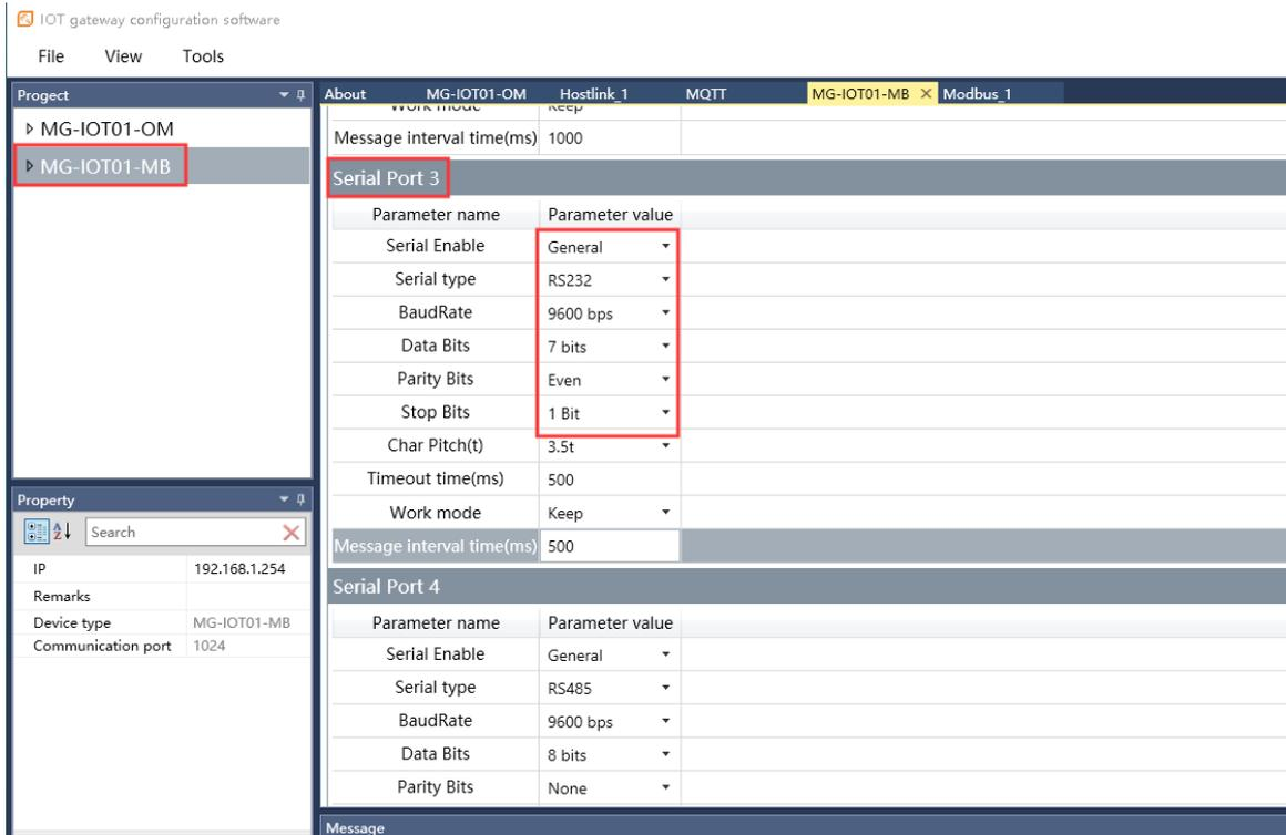
Configure the collection channel parameters as shown below:
