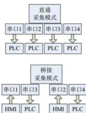
In Bridge mode, PLC data is collected without affecting HMI and PLC communication. The connection method is HMI and PLC respectively connected to the two serial ports of the gateway (serial port 1 and serial port 3 are one group, serial port 2 and serial port 4 are One group, serial port 1, 2 to HMI, serial port 3, 4 to PLC). The HMI data enters the gateway through the serial ports 1, 2, and enters the PLC from the serial ports of the gateways 3 and 4.
