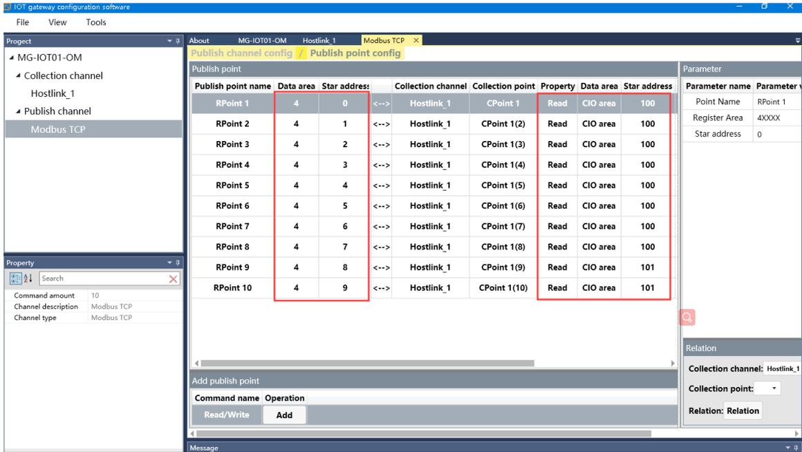
After completing the above settings, the Modbus TCP client can use the Modbus TCP protocol to access the gateway through the gateway IP address 192.168.1.254 and Modbus data communication port 502 to access the collected data. This document uses Modbus Poll to simulate Modbus TCP client to collect data.
