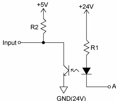
When Port A is supplied 24V from an external input port, the input is recognized to 5V(High).
