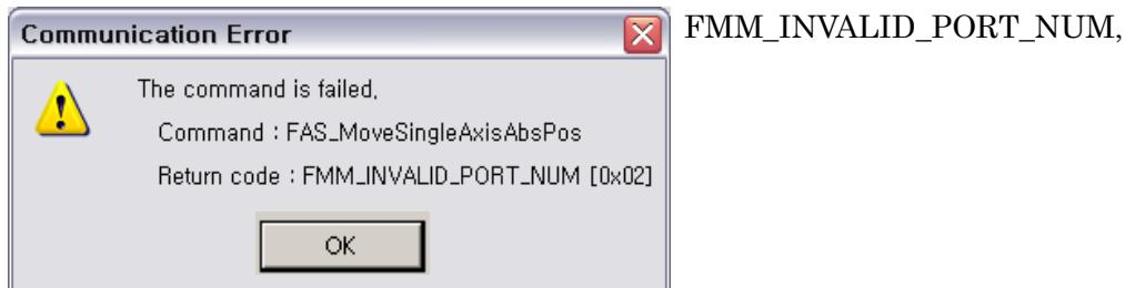
COM Port number is not exist. Checking the 'Device Manager' window in Window OS.
