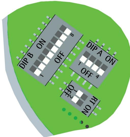
Figure 3: DIP switches
