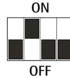
Set the baud rate to 115200 bits per second and Even parity bit:
