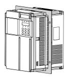
b. Fasten the AC drive with the bracket mounted onto the mounting backplate of the control cabinet.
