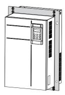
b. Fasten the AC drive onto the backplate of the control cabinet from the front of the control cabinet.
