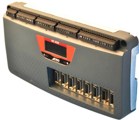
It is designed to be configured and programmed for the application using a PC running Trio's *Motion Perfect* application software, and then may be set to run "standalone" if an external computer is not required for the final system. Programs and data are stored directly to **FLASH** memory, thus eliminating the need for battery backed storage.
