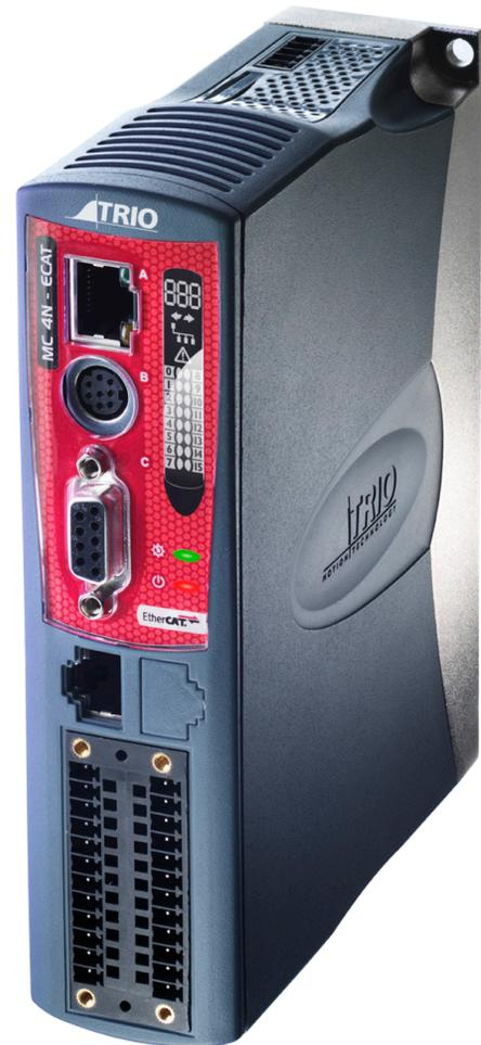
The MC4N-ECAT has one built in RS232 port and one built in duplex RS485 channel for simple factory communication systems. Either the RS232 port or the RS485 port may be configured to run the Modbus or Hostlink protocol for PLC or HMI interfacing.
