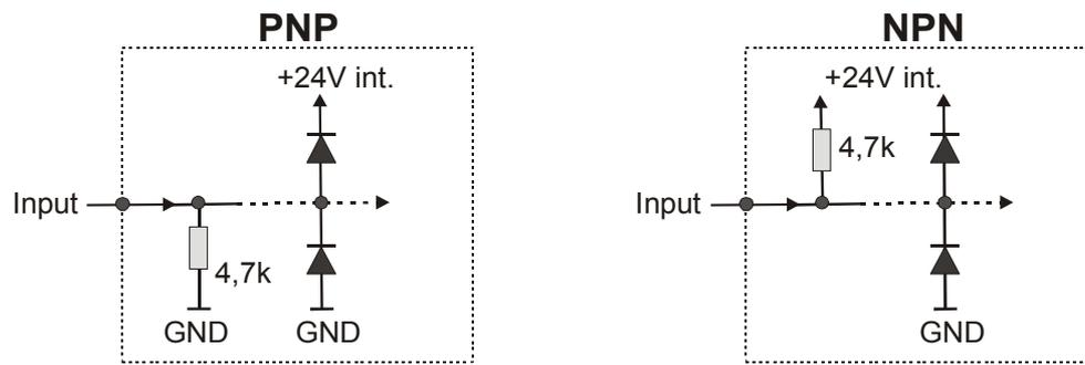
The counting inputs A and B are designed for input frequencies up to 100 kHz (with all counter modes) and up to 25 kHz (with all other operating modes). The minimum pulse duration on the Reset input must be 500 µsec. (maximum frequency 1 kHz)
