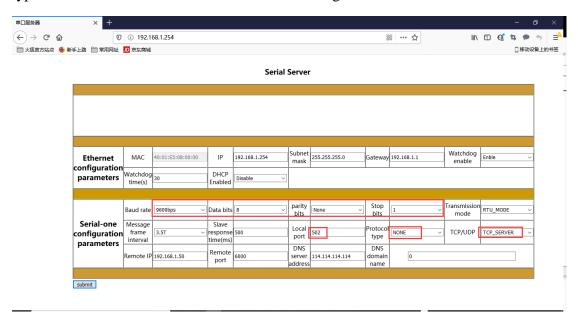
Open the TCP debug assistant, simulate the TCP Client, and access the protocol converter 192.168.1.254 port 502.
