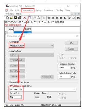
Open Modbus Slave (simulated serial port device), click Connection or press F3 shortcut key, set the correct serial port number and communication parameters in the pop-up window, and click OK.
