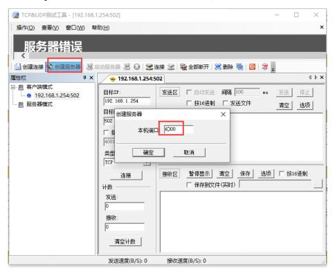
Mouse over the server mode to confirm the native, and then click to enable the server. The protocol converter IP and port number will be displayed after successful
