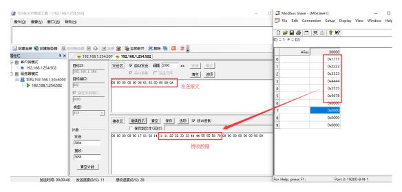
5.When testing ODOT-S2E1, if the protocol converter USES TCP\_CLINET mode (only one server is supported) and communicates with COM1 and COM2 at the same time, set the remote port number of COM1 and COM2 to the same port number 6000 and the local port number to a different port number 502/503 on the configuration page.
