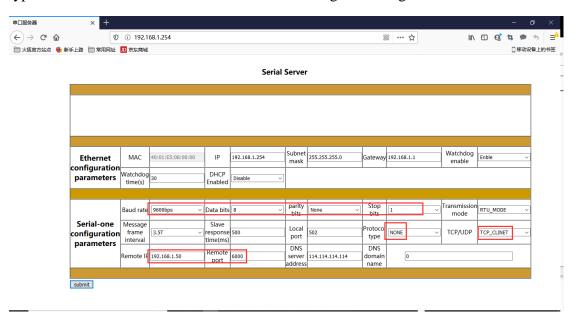
Open the TCP debugging assistant, simulate THE TCP Server (native IP address 192.168.1.50, port number 6000), and wait for the protocol converter to actively connect.
