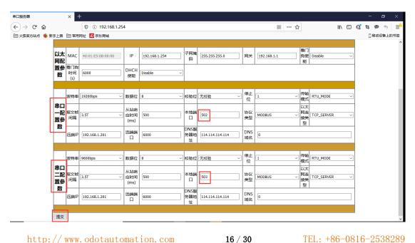
The data of serial port 1 or serial port 2 are distinguished by the port number at MODBUS TCP. For example, to read data of serial port 1, set the host computer software port number of Modbus TCP/IP terminal to 502, and set the port number of serial port 2 to 503 when reading data of serial port 2.
