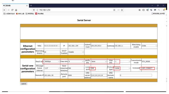
Open the TCP debugging assistant to simulate the UDP connection protocol converter. Open the Serial Port Utility to simulate the underlying Serial Port device. The following figure shows the screenshot of normal communication of data:
