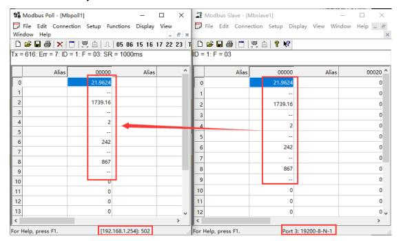
5. When testing ODOt-S2E1, there are two serial ports. When serial port 1 and serial port 2 are used at the same time, please set different local port Numbers, otherwise the module will recognize COM1 and COM2 as the same port. The diagram below:
