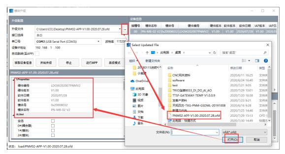
Select 0# coupler, tick " $\sqrt{}$ ", click to start upgrading, and click to run APP after completion. Or select automatic jump (to APP) and click to start the upgrade.
