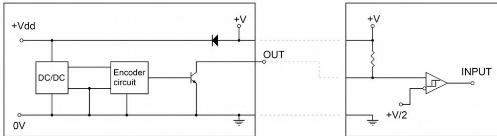
4.13 Recommended circuit, parallel output with Push-Pull drive (PY code)
