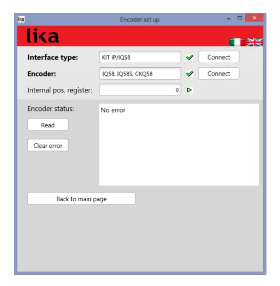
If an error occurs and the system is not able to solve it after pressing the **CLEAR ERROR** button, please take note of the error code that appears in the window and reach Lika Electronic's After Sales and Technical Service.
