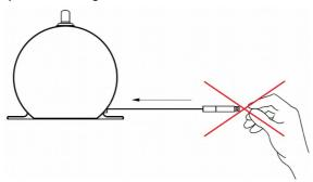
Always keep the wire aligned not to damage the equipment (maximum deviation: 3°).
