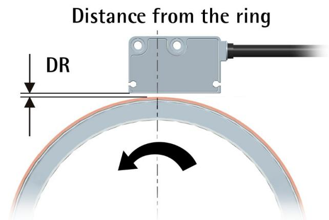
Figure 5 - Sensor / ring mounting gap
