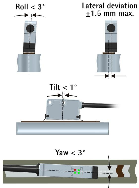
Figure 2 - Sensor / scale mounting tolerances
