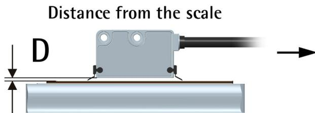
Figure 1 - Sensor / scale mounting gap
