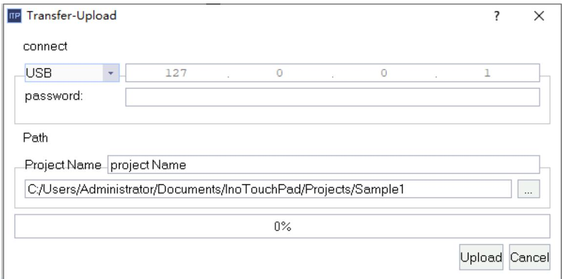
Select the connection method and input the IP address of the connected HMI:
