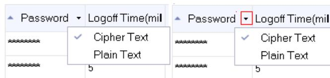
Logoff Time (min): If the the user does not perform any operation after this time, the user will be automatically logged out (the defalut is 5 min). If you set it to 0, automatic logout is disabled.
