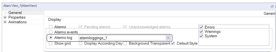
Figure 9-9 Alarm log configuration
